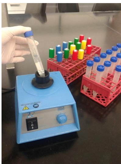
Figure 2.10: Cells detachment by vortexing with glass beads.
