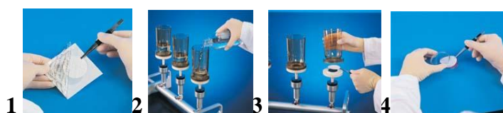
Figure 2.5: Membrane filter method procedure.
