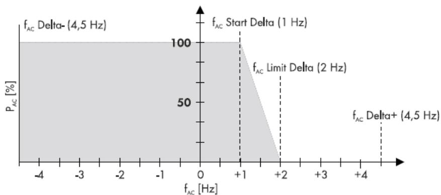
Figure 2.2 Frequency Shift Power Control (SMA America, 2011)
