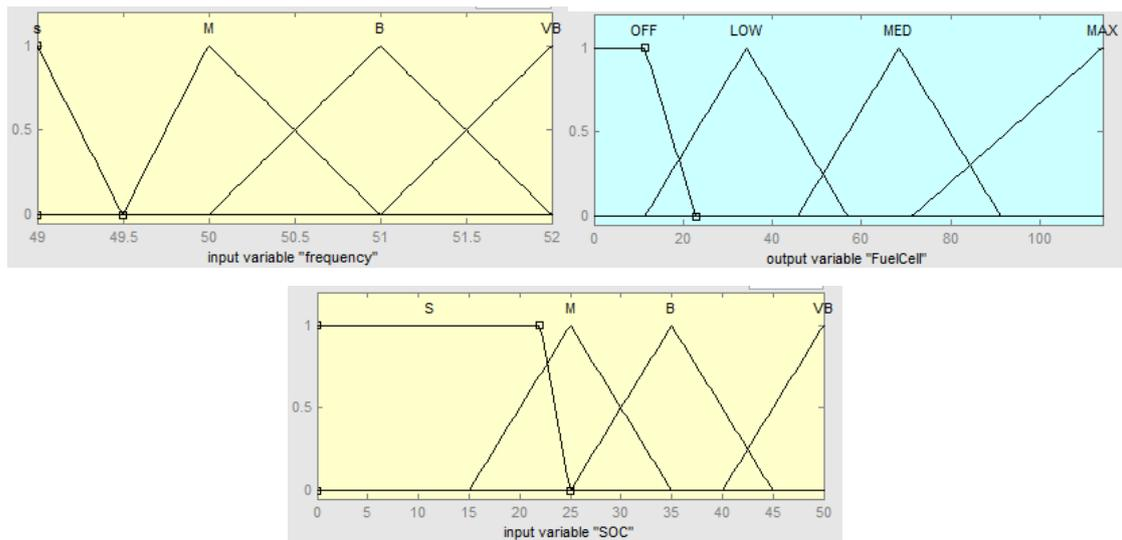
Figure 5.6 Membership functions for FLS 3
