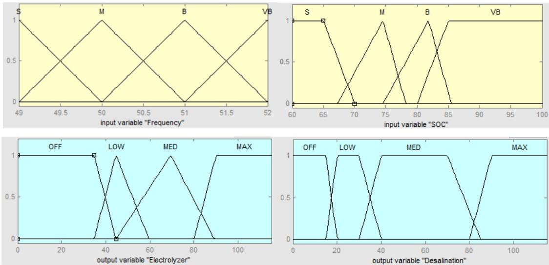
Figure 5.5 Membership functions for FLS 2
