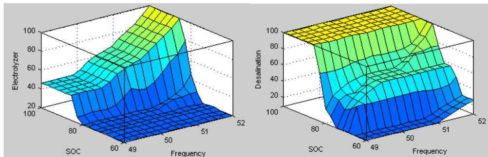
Figure 5.8 Control Surfaces for FLS 2
