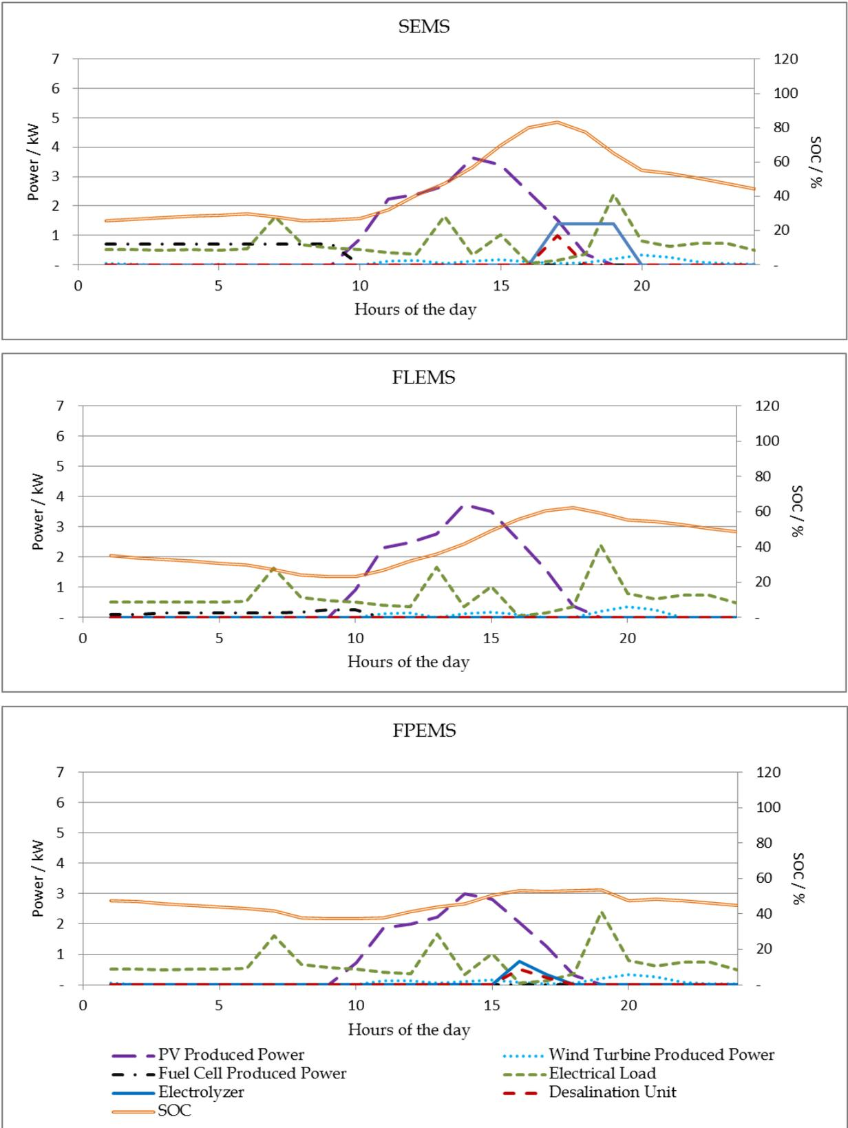
Figure 6.13 Hourly produced and consumed power from the different microgrid components for the 10th of December
