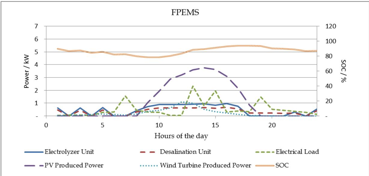
Figure 6.12 Hourly produced and consumed power from the different microgrid components for the 1st of October
