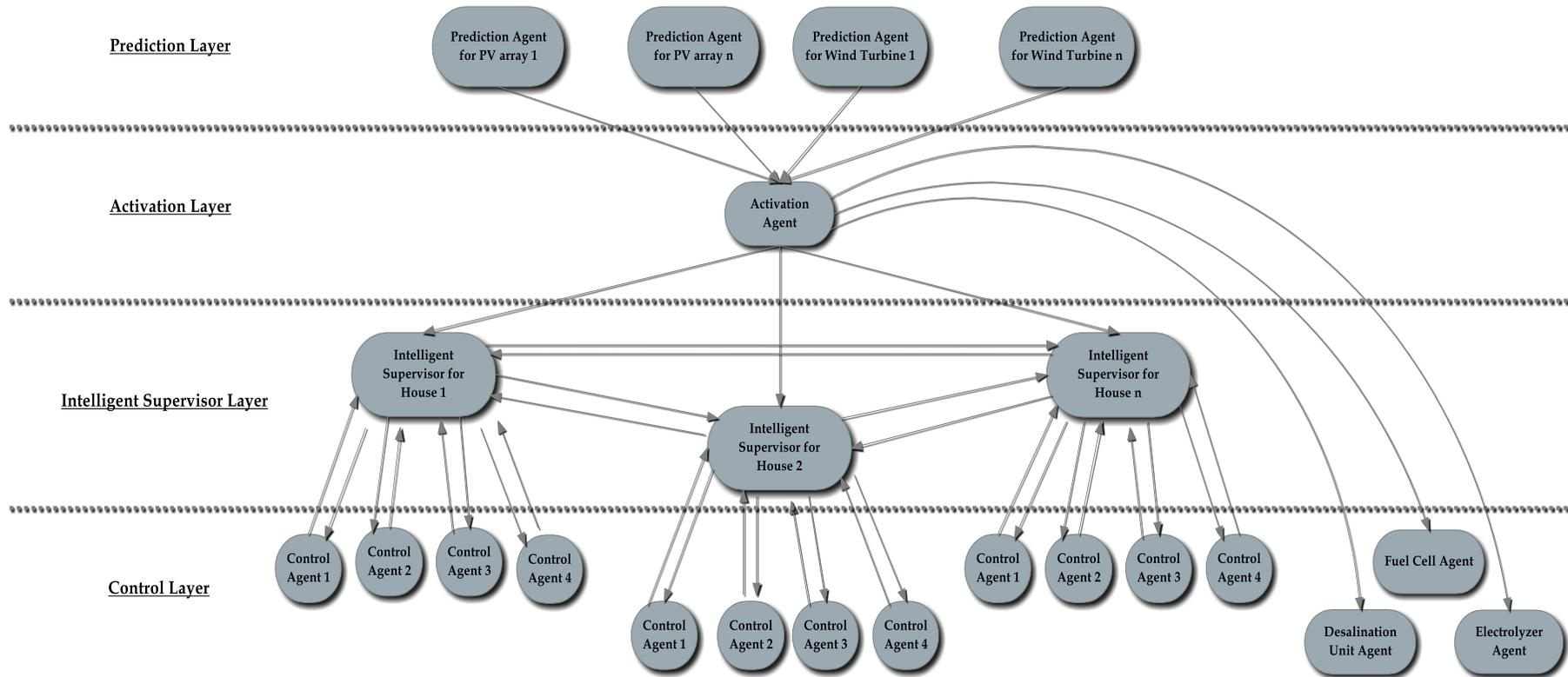
Figure 7.4 Intelligent Demand Side Management System structure
