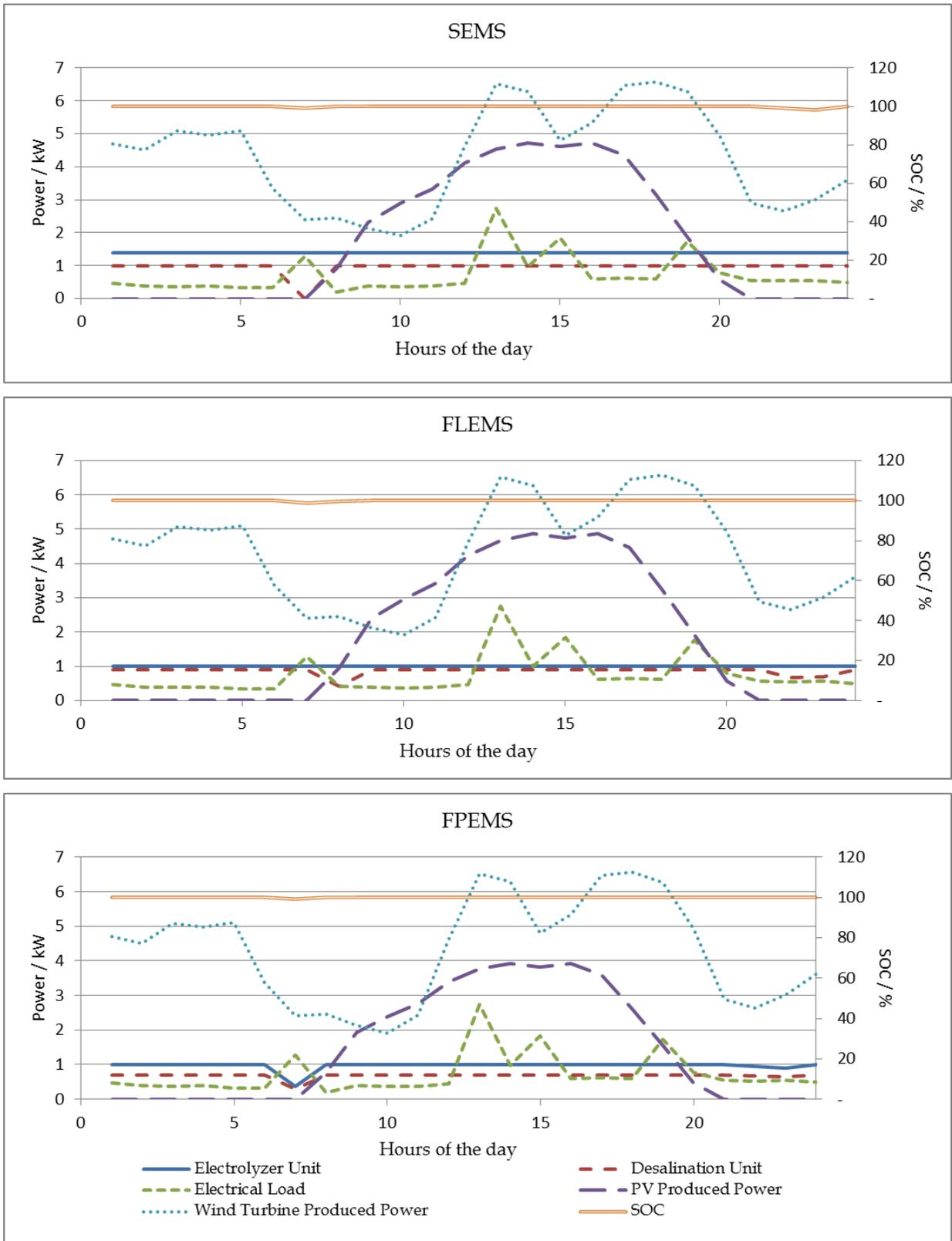
Figure 6.11 Hourly produced and consumed power from the different microgrid components for the 1st of August
