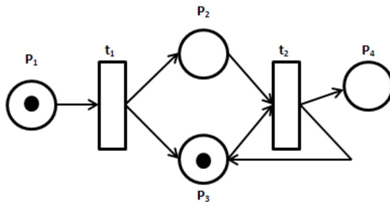
Figure 4.5 A typical petri net graph
