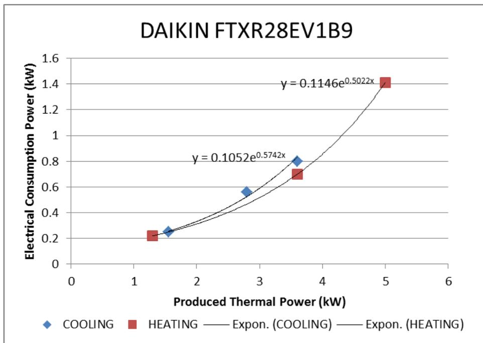
Figure 6.1 Operational characteristics of air conditioning unit
