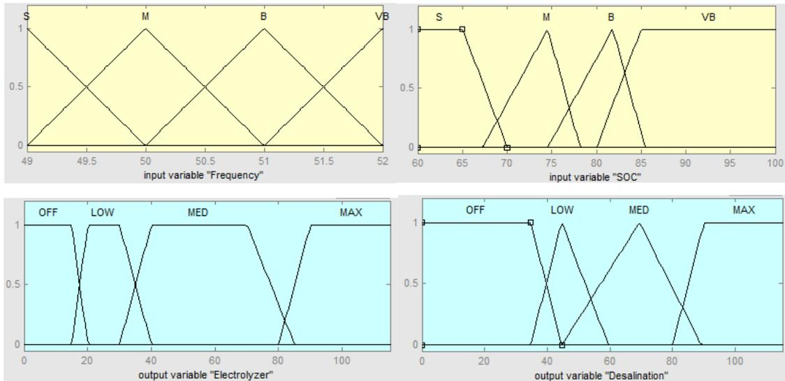
Figure 5.4 Membership functions for FLS 1
