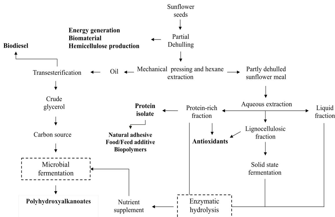
**Figure 2.7** Advanced sunflower-based biorefinery concept
