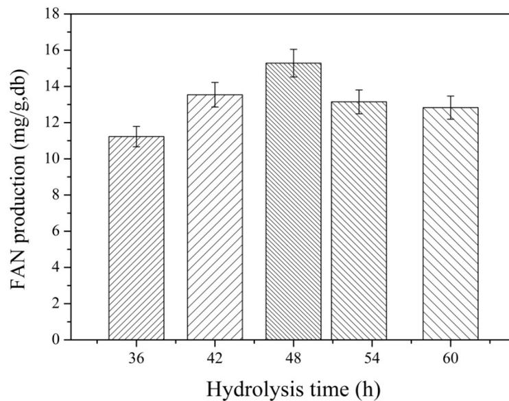
**Figure 5.9** Effect of time course of SSF on FAN production during hydrolysis of 45 g/L initial solid concentration (SFM and remaining SSF solids)
