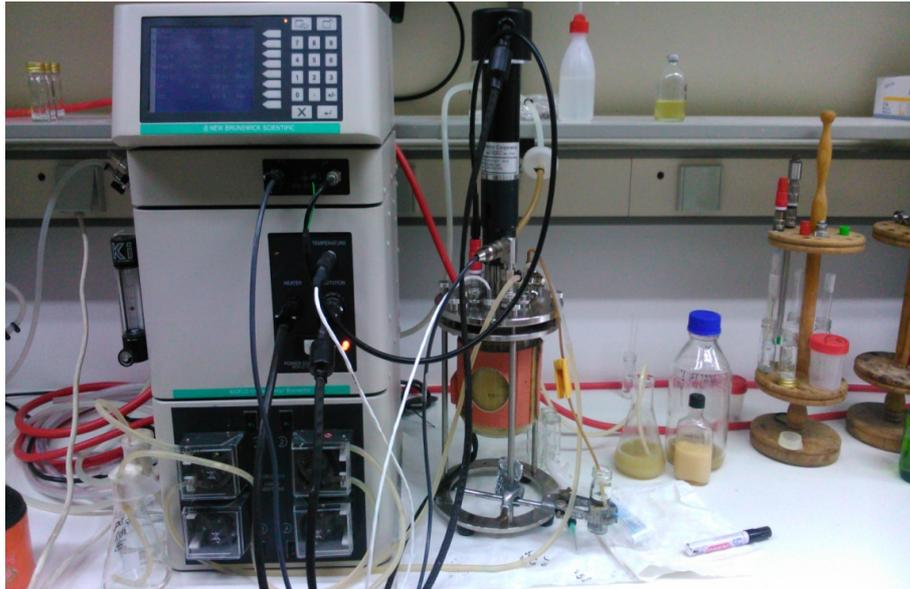
**Figure 4.2** Bioreactor employed in bacterial bioconversions
