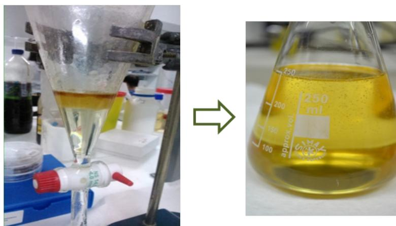
**Figure 5.1** Crude glycerol decanting in separation funnels
