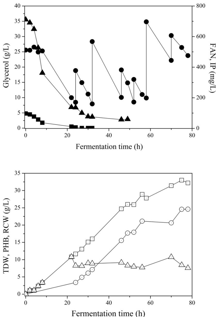
**Figure 6.8** Profile change of glycerol (●), FAN (▲), IP (■), TDW (□), PHB (○) and RCW (Δ) during fed-batch bioreactor fermentation of *C. necator* on sunflower meal hydrolysate with an initial FAN concentration of 710 mg/L (C/FAN ratio of 14.05 g/g)
