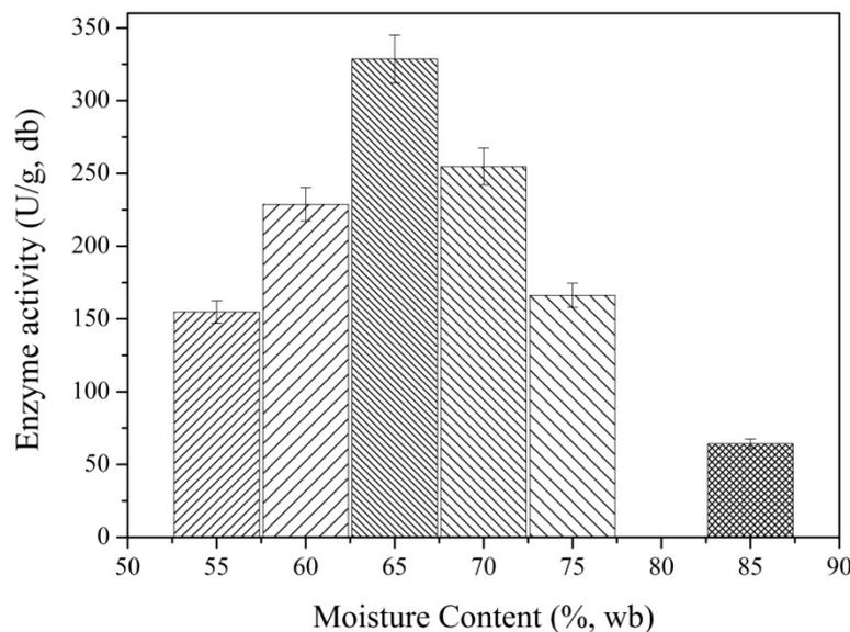
**Figure 5.2** Enzymatic activities in different initial moisture contents at 48 h of SSF
