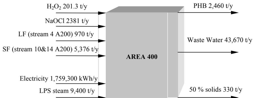
**Figure 10.9** Summary of total quantities of input and output streams for PHB recovery including the production of lytic enzymes (AREA 400)
