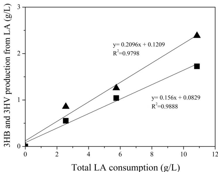
**Figure 7.1** Production of 3HB and 3HV during shake flask fermentations of *C. necator* carried out on crude glycerol and sunflower meal hydrolysate at different supplementations of levulinic acid (▲) 3HV, (■) 3HB
