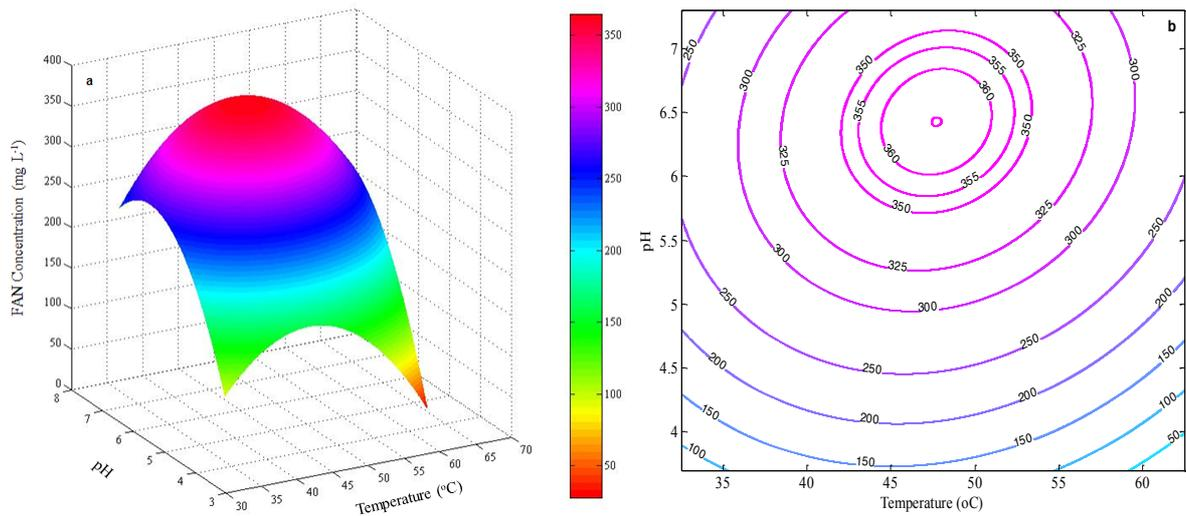
**Figure 9.3** Graphical representation of the model predictions for the response variable  $Y_1$  (FAN concentration) for the entire range of parameter values as a 3D graph (a) and as a counter plot (b)
