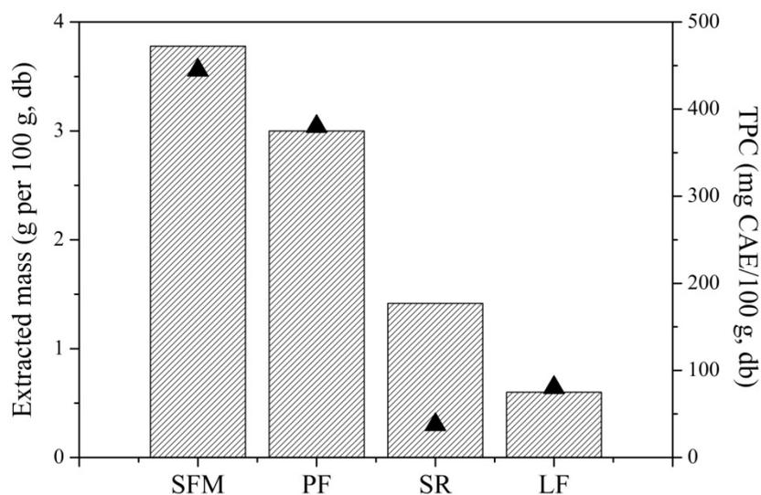
**Figure 8.4** Total Phenolic Content (TPC) measured by the Folin-Ciocalteu method and total quantity of material extracted from various streams including sunflower meal (SFM), protein-rich fraction (PF), lignocellulose-rich fraction (LF) and solid residue (SR)
