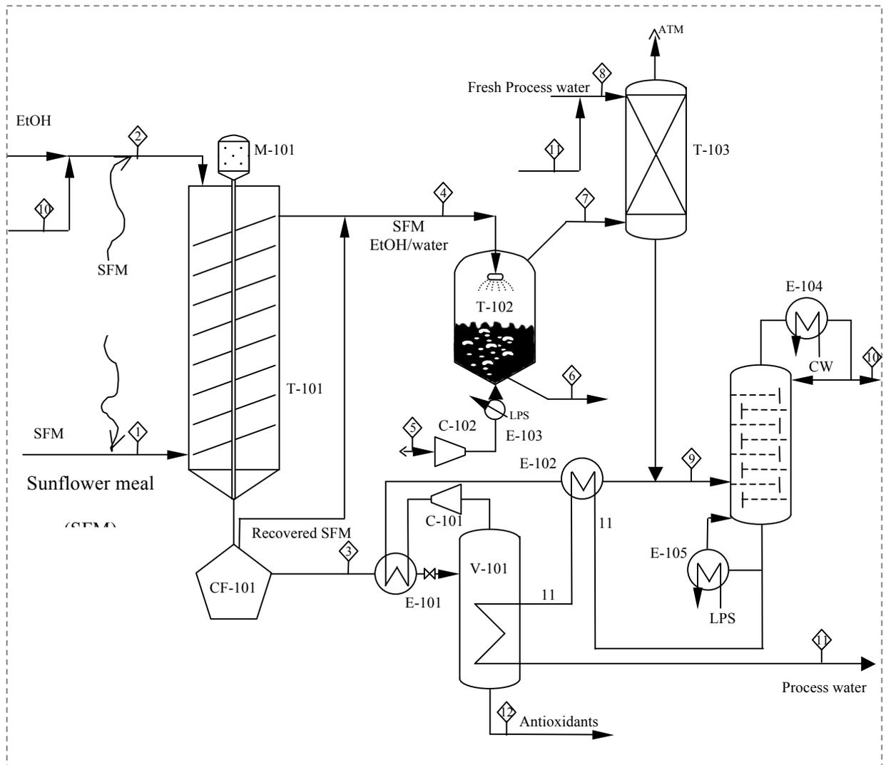
**Figure 10.2** Process flow diagram for AREA 100: antioxidants extraction
