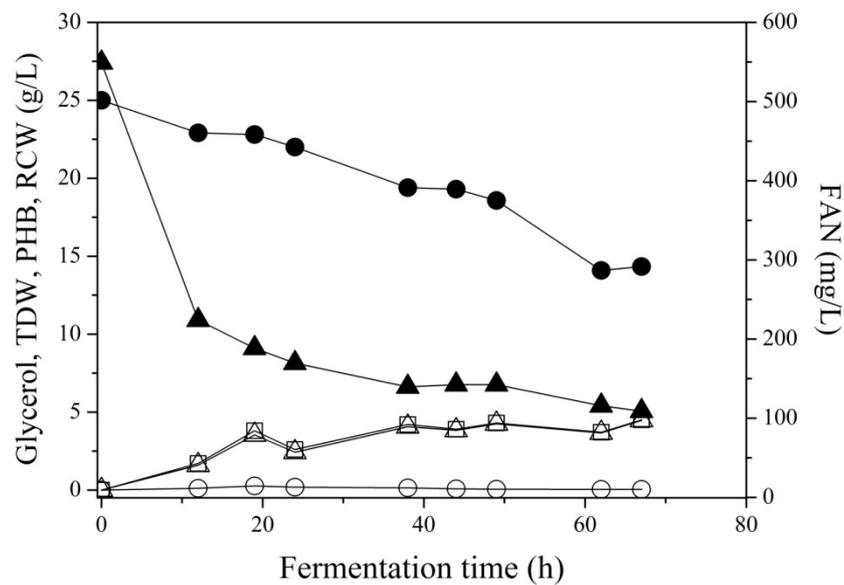
**Figure 6.1** Profile change of FAN (▲), glycerol (●), TDW (□), PHB (○) and RCW (Δ) concentration during shake flask fermentation of *C. necator* DSM 11348 on SFM hydrolysate and crude glycerol.
