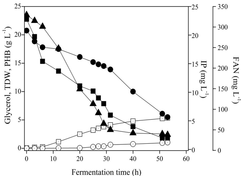
**Figure 9.7** Consumption of FAN (○), IP (Δ) and glycerol (□) as well as production of TDW (■) and PHB (▲) during shake flask fermentation of *C. necator* cultivated on crude glycerol and the lysate obtained by the enzymatic lysis of non-PHA cell mass
