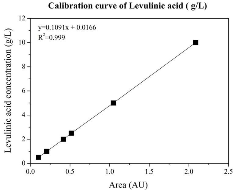
**Figure 4.8** Calibration curve of Levulinic acid
