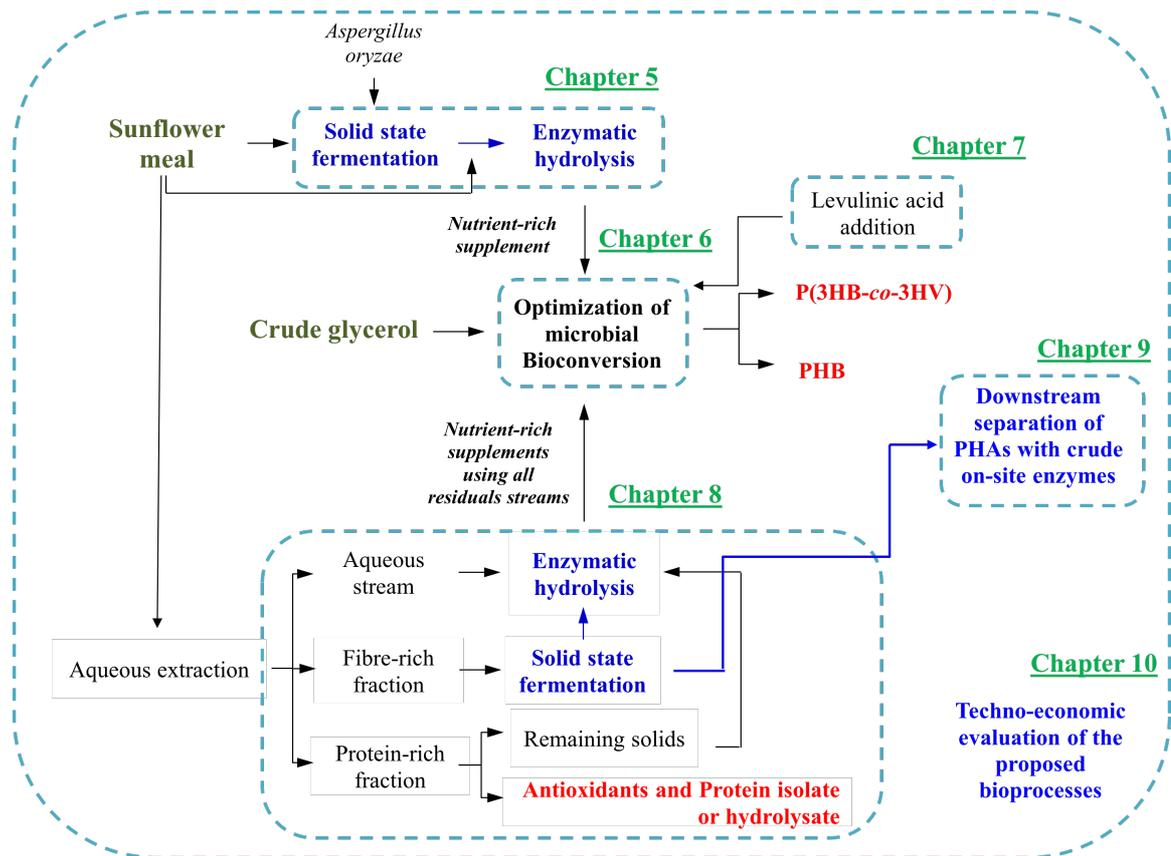
**Figure 3.1** Overview of the experimental process designed during the present study for the valorisation of SFM and crude glycerol towards the development of an advanced biorefinery concept
