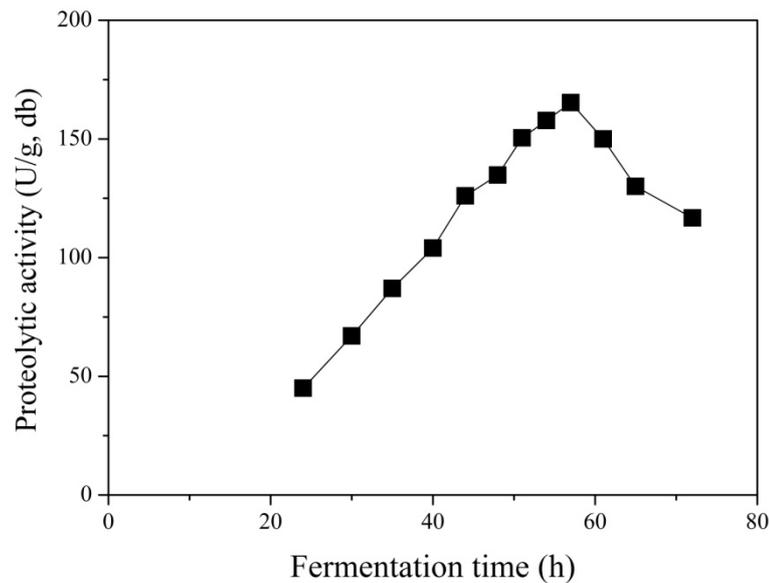
**Figure 8.6** Proteolytic activity produced during SSF with *A. oryzae* carried out on lignocellulose-rich fraction
