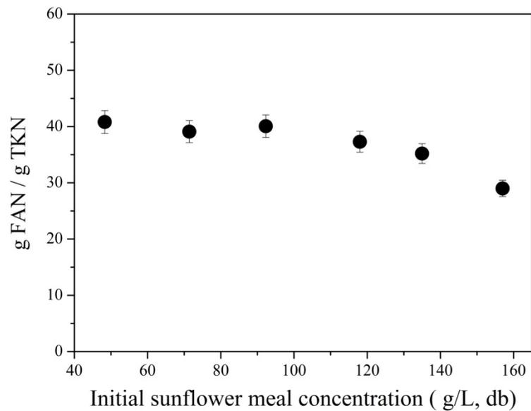
**Figure 5.11** Overall TKN to FAN conversion yield at different total SFM concentrations used for both SSF and hydrolysis stages
