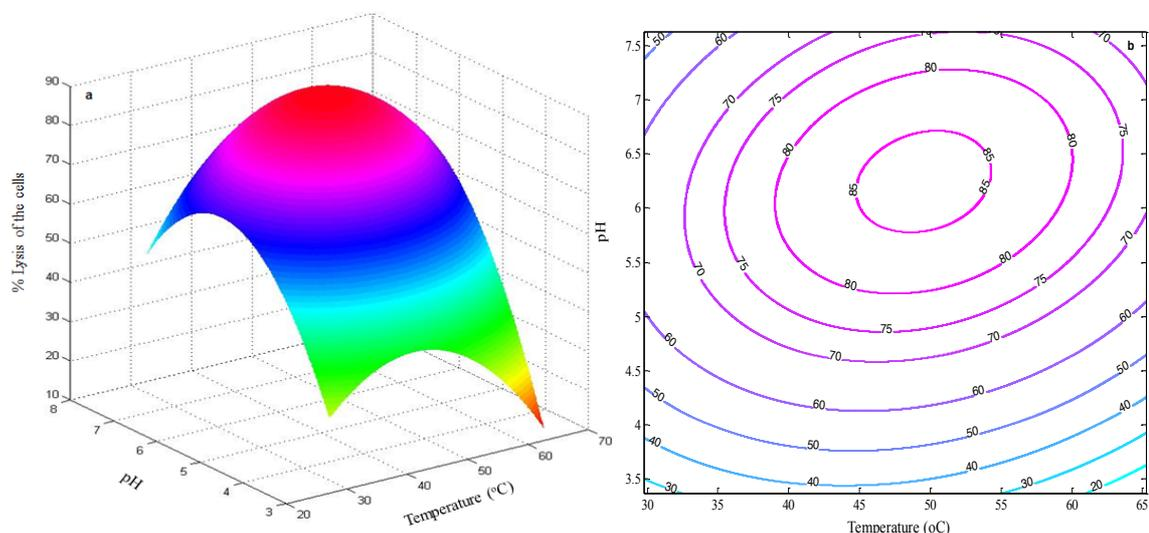
**Figure 9.4** Graphical representation of the model predictions for the response variable  $Y_2$  (percentage of non-PHA cell lysis) for the entire range of parameter values as a 3D graph (a) and as a counter plot (b)
