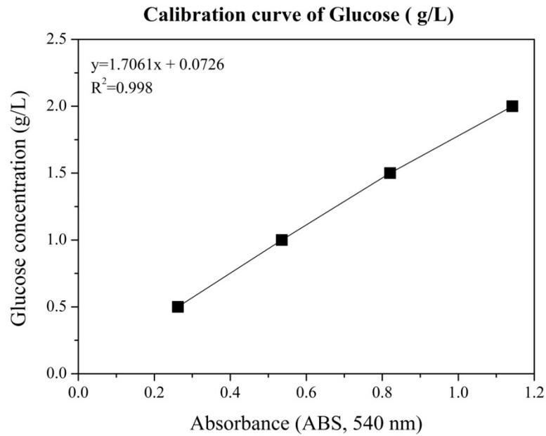
**Figure 4.5** Calibration curve of glucose
