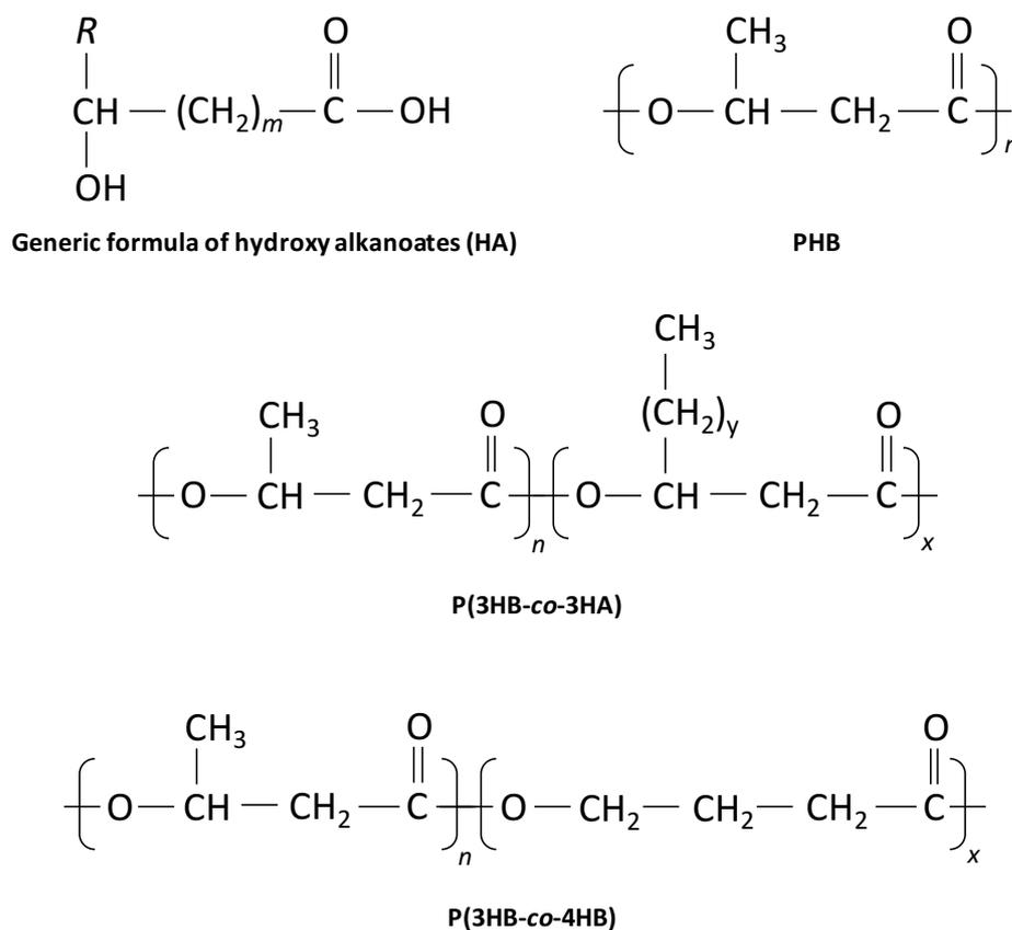
**Figure 2.4** Generic chemical formula of HA monomers and common PHA copolymers
