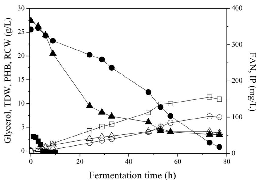
**Figure 6.4** Profile change of FAN (▲), IP (■) glycerol (●), TDW (□), PHB (○) and RCW (Δ) during shake flask fermentation of *C. necator* DSM 7237 on SFM hydrolysate and pre-treated crude glycerol with a purity of 92.4 % (w/w).
