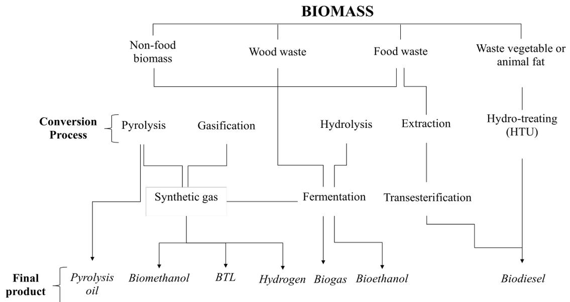
**Figure 2.1** Pretreatment methods implemented in biofuels production (Adapted from Stöcker, 2008)
