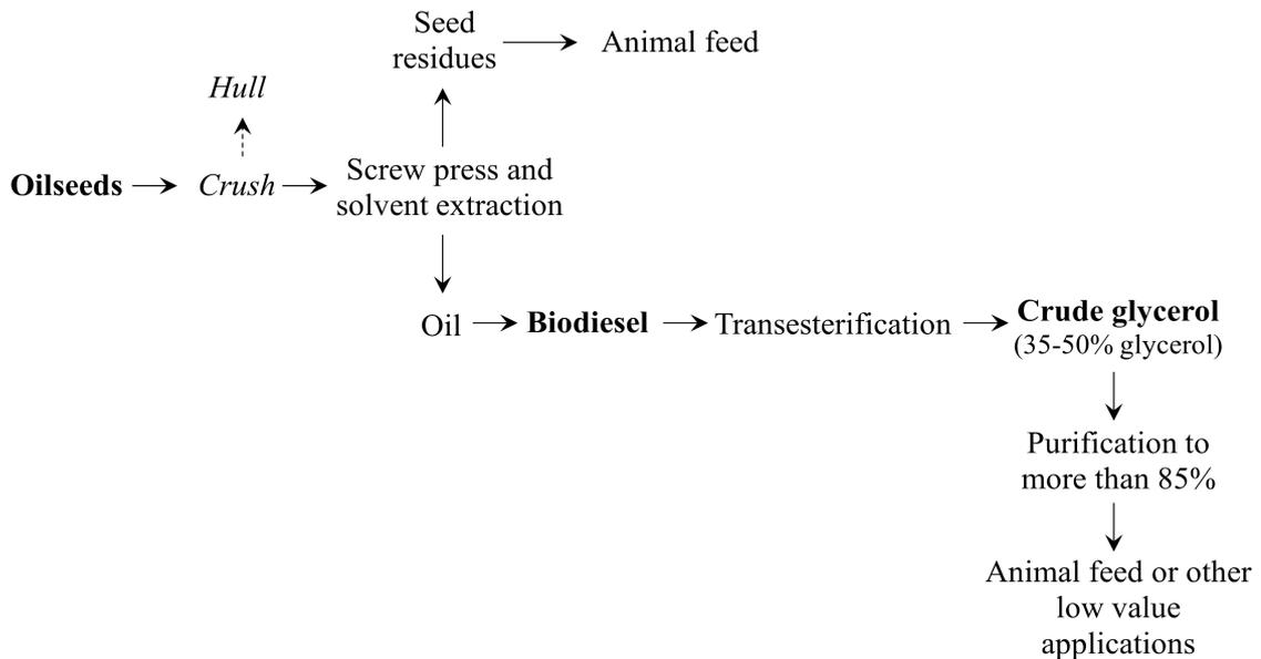
**Figure 2.3** Biodiesel production process from oilseeds
