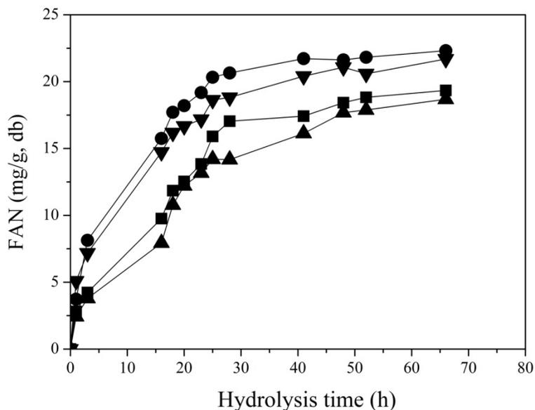
**Figure 5.13** FAN production during SFM hydrolysis at different initial proteolytic activities (▲: 3.2 U/mL, ■: 6.4 U/mL, ▼: 9.6 U/mL, ●: 16.4 U/mL) using the same initial SFM concentration of 102 g/L (db)
