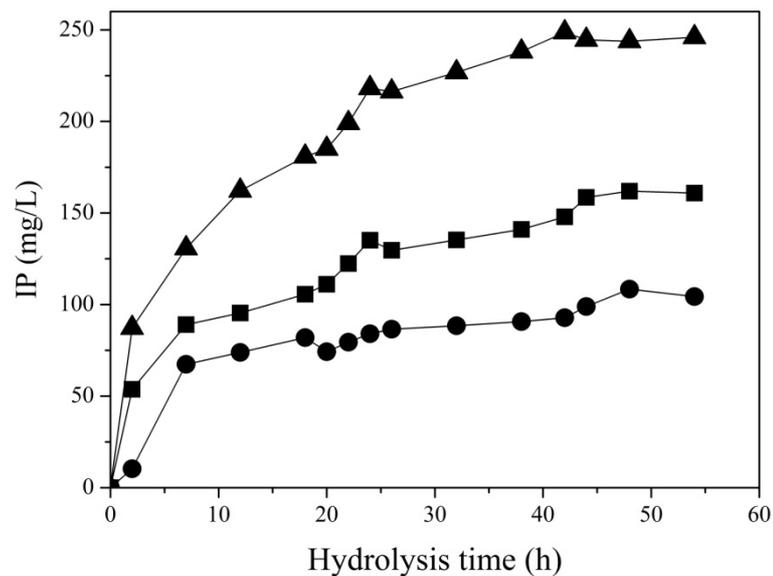
**Figure 5.12** IP production during solid (SFM and remaining SSF solids) hydrolysis at initial solid concentrations of 46.3 g/L (●), 70.4 g/L (■) and 92.2 g/L (▲) using an initial enzyme activity of 6.4 U/mL
