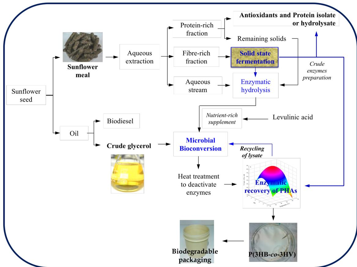
**Figure 9.1** Advanced sunflower-based biorefinery including the use of crude enzyme consortia for downstream separation of PHB and P(3HB-*co*-3HV)
