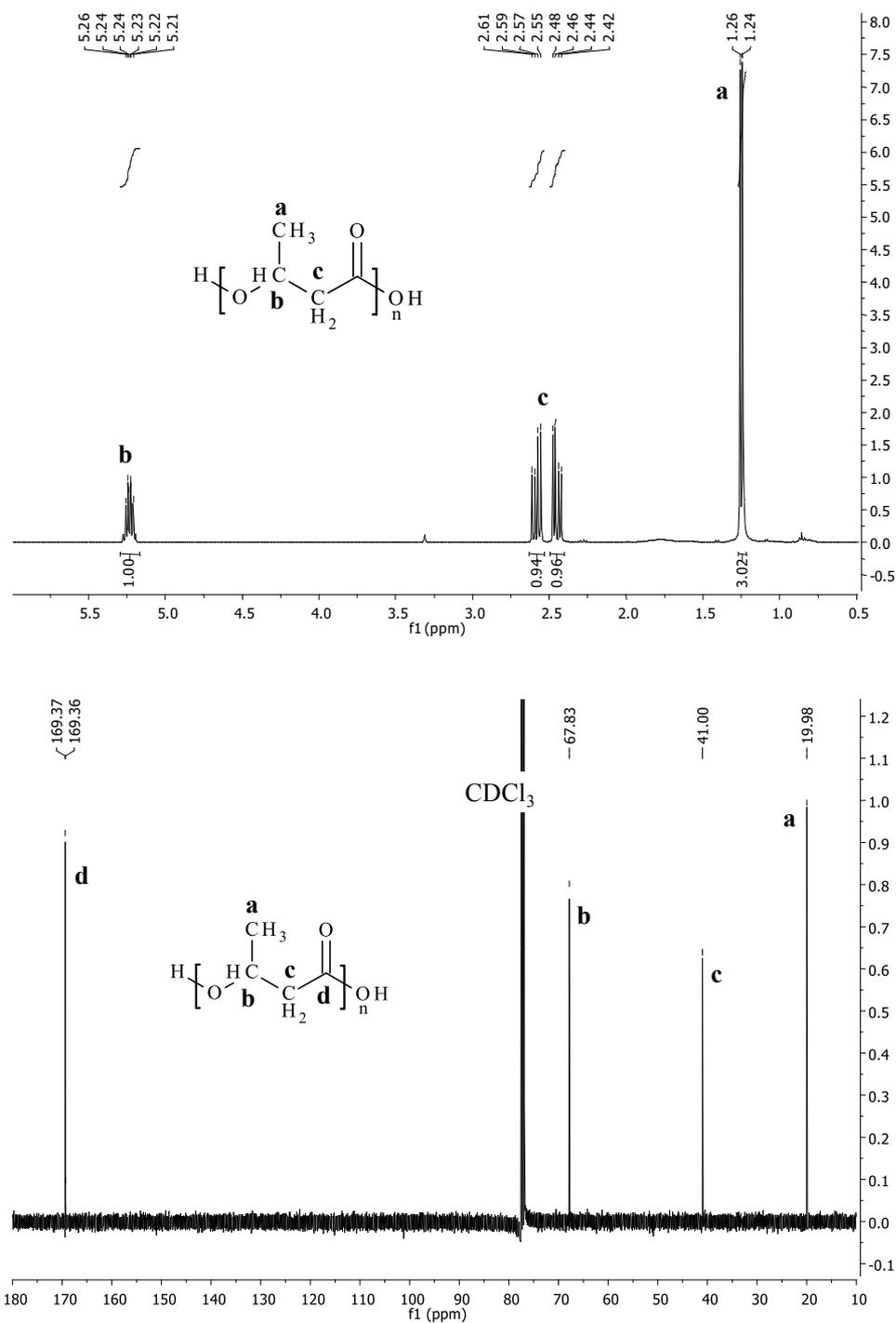
**Figure 7.4:**  $^1\text{H}$  NMR spectrum (a) and  $^{13}\text{C}$  NMR spectrum (b) of PHB produced from sunflower meal hydrolysates and crude glycerol
