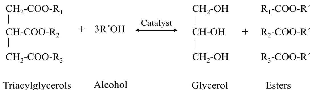
**Figure 2.2** Transesterification reaction of triglycerides with base catalyst to produce esters and glycerol
