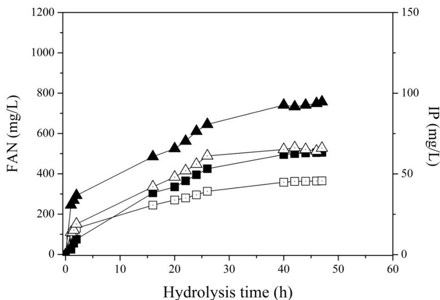
**Figure 8.7** FAN and IP production during enzymatic hydrolysis of 50 g/L ( $\square$ , FAN;  $\Delta$ , IP) and 100 g/L ( $\blacksquare$ , FAN;  $\blacktriangle$ , IP) initial concentration of solids from the lignocellulose-rich fraction
