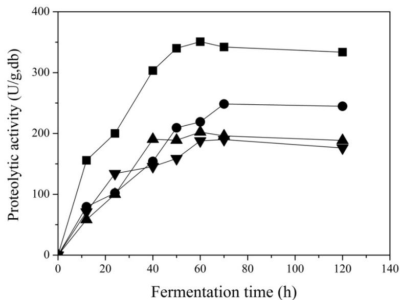
**Figure 5.4** Proteolytic activity during SSF with *A. oryzae* carried out at four different pH values (■: natural, ●: 6.5, ▲: 5.5, ▼: 4.5) with 65 % initial moisture content
