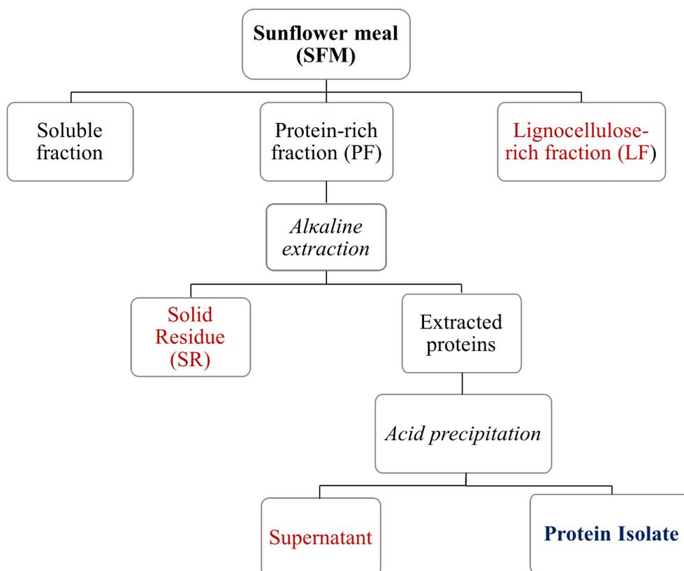
**Figure 4.1** SFM fractionation protocol followed for the production of protein isolate (adapted by Villaneuva et al. 1999)
