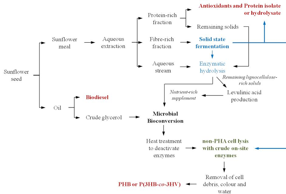
**Figure 8.1** Sunflower-based biorefinery concept: Utilization of SFM for the production of antioxidants, protein isolate and PHB or P(3HB-co-3HV)
