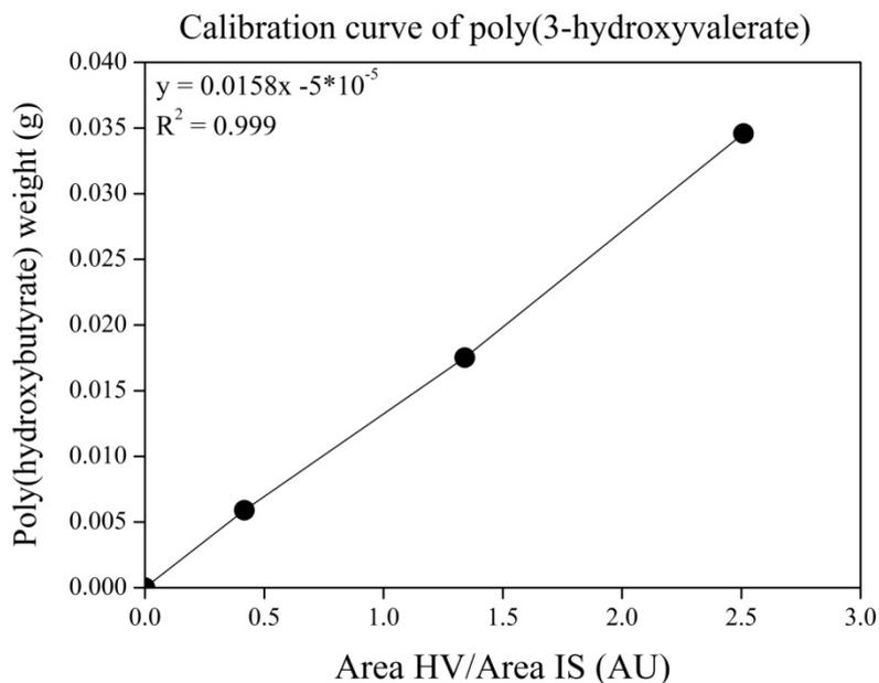
**Figure 4.11** Calibration curve of P(3-hydroxyvalerate) with internal standard (benzoic acid)
