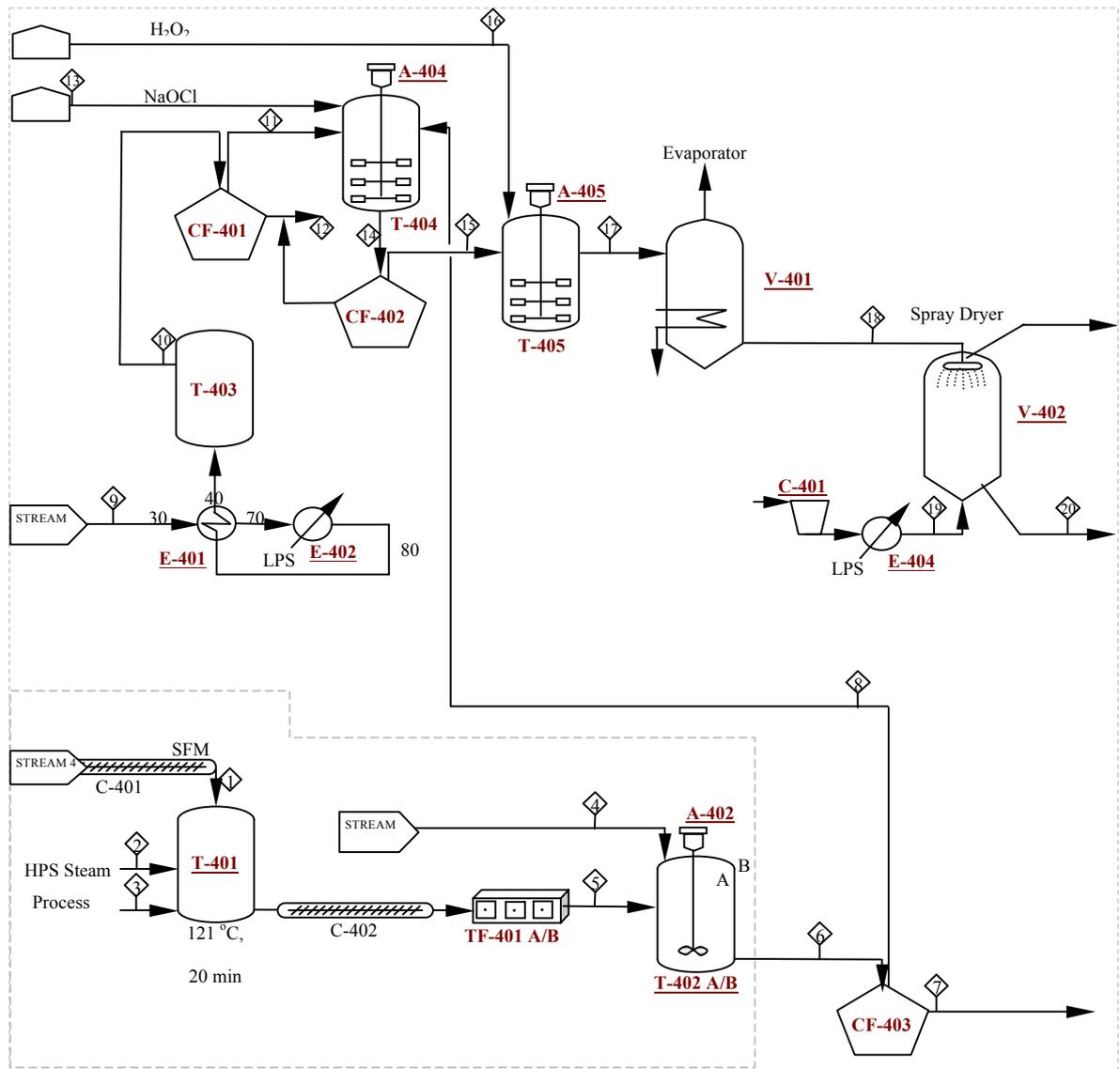
**Figure 10.8** Process flow diagram for AREA 400: Production of crude enzyme-rich extract and PHB recovery
