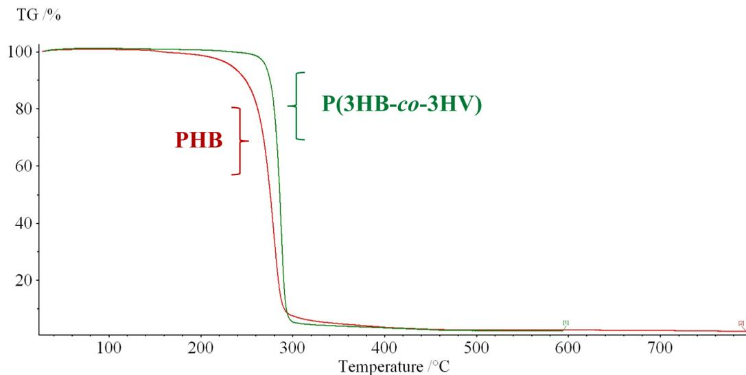
**Figure 7.6:** Thermogravimetric analysis curve for PHB and P(3HB-*co*-3HV) produced from sunflower meal hydrolysates and crude glycerol
