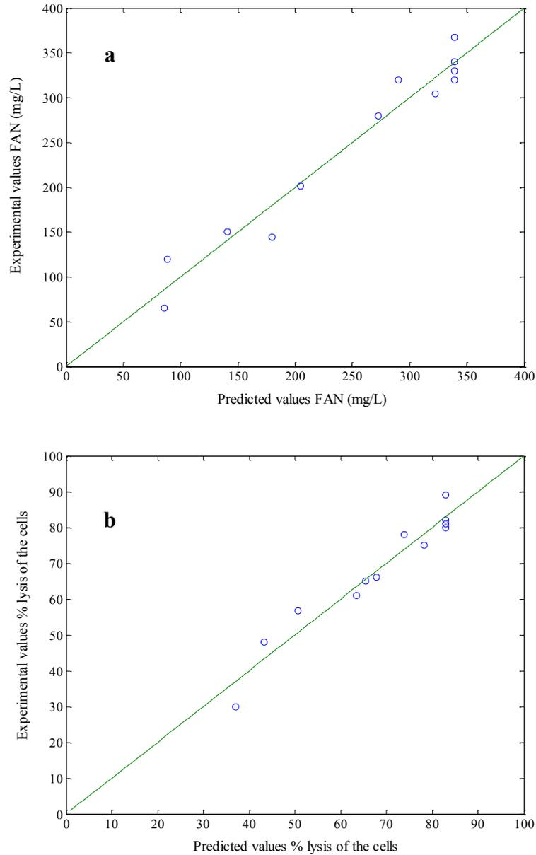
**Figure 9.2** Predicted values versus experimental results of FAN production (a) and of percentage of cell lysis (b)
