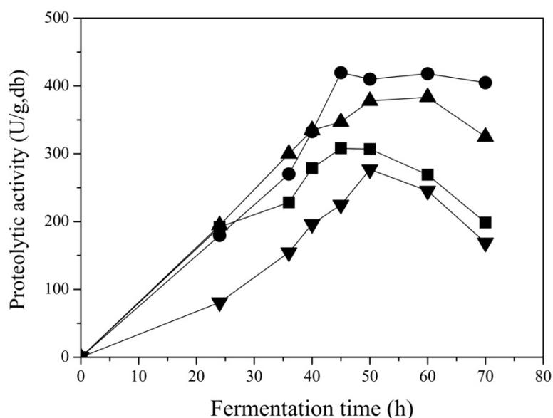
**Figure 5.3** Proteolytic activity during SSF with *A. oryzae* carried out at four different initial moisture contents (■: 60 %, ●: 65 %, ▲: 70 %, ▼: 75 %)
