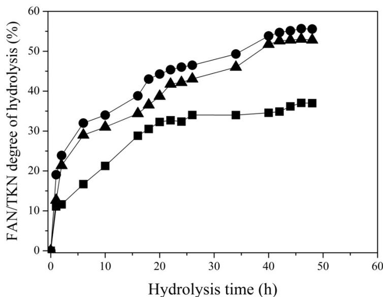
**Figure 8.3** Degree of hydrolysis expressed as increasing FAN to TKN ratio during hydrolysis of protein isolate utilizing different initial proteolytic activities of crude enzyme consortia produced via SSF carried out with *A. oryzae*. (■) 6 U/mL, (▲) 24 U/mL, (●) 30 U/mL
