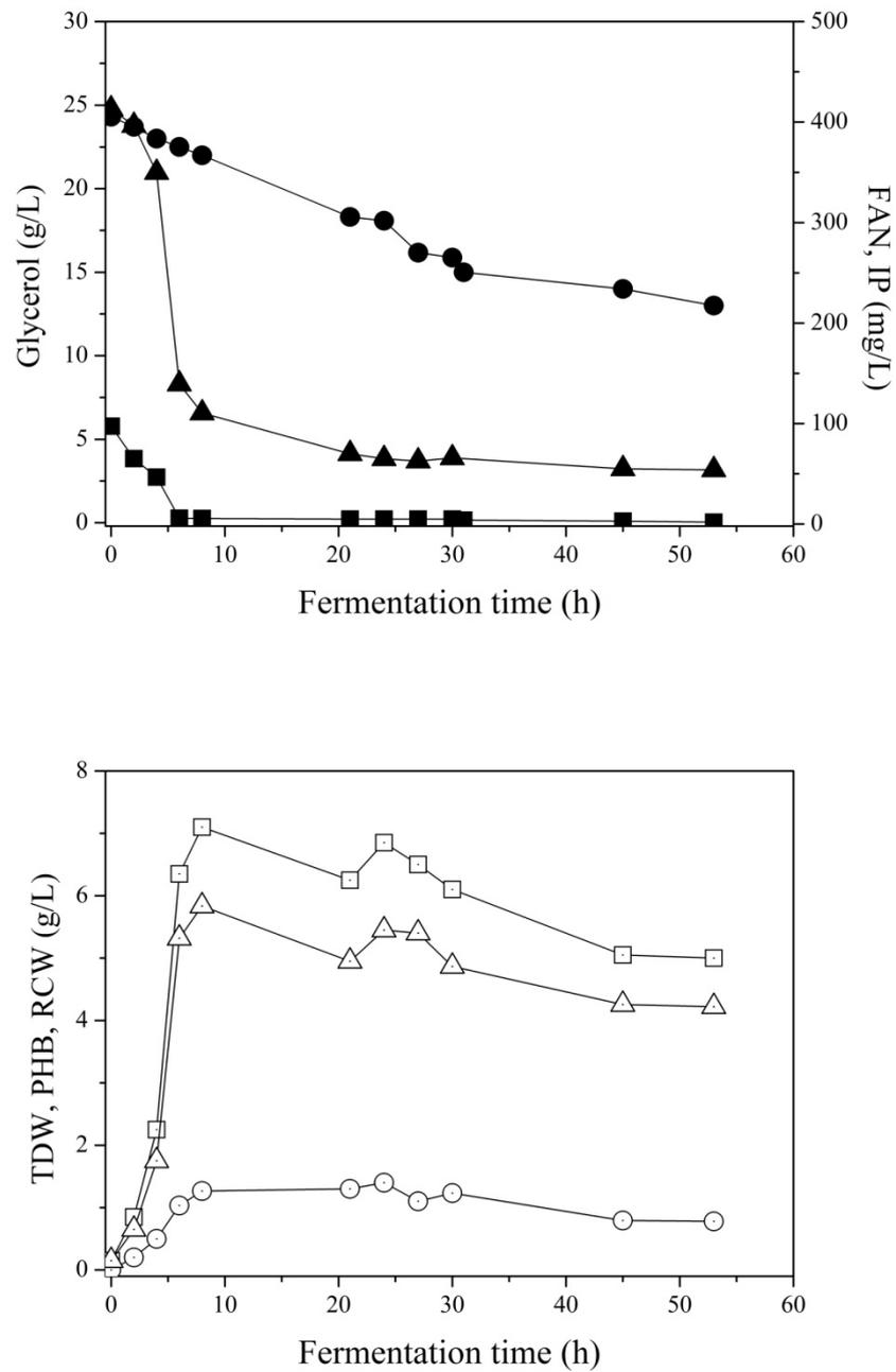
**Figure 8.9** Profile change of FAN (▲), glycerol (●), IP (■), TDW (□), PHB (○) and RCW (Δ) during batch bioreactor fermentation of *C. necator* cultivated on crude glycerol and Hydrolysate I (obtained from the lignocellulose-rich fraction)
