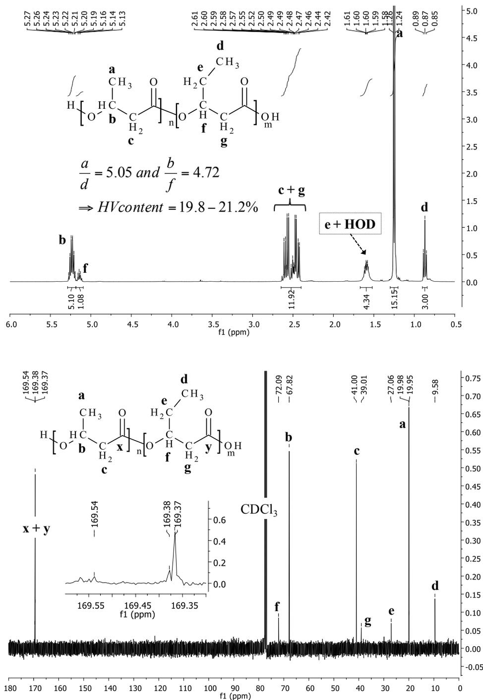
**Figure 7.5:** <sup>1</sup>H NMR spectrum (a) and <sup>13</sup>C NMR spectrum (b) of produced P(3HB-co-3HV) from sunflower meal hydrolysates, crude glycerol and levulinic acid
