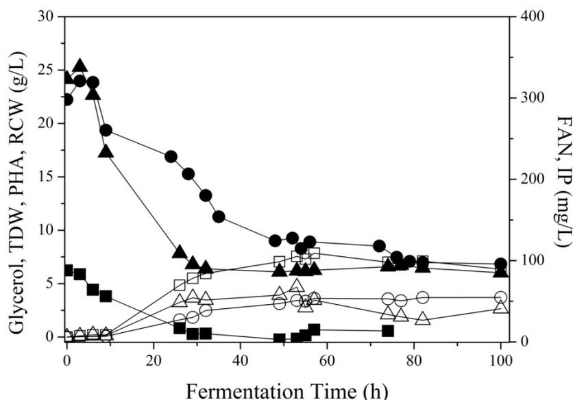
**Figure 6.3** Profile change of FAN ( $\blacktriangle$ ), IP ( $\blacksquare$ ) glycerol ( $\bullet$ ), TDW ( $\square$ ), PHB ( $\circ$ ) and RCW ( $\Delta$ ) during shake flask fermentation of *C. necator* DSM 7237 on SFM hydrolysate and original crude glycerol with a purity of 91 % (w/w).
