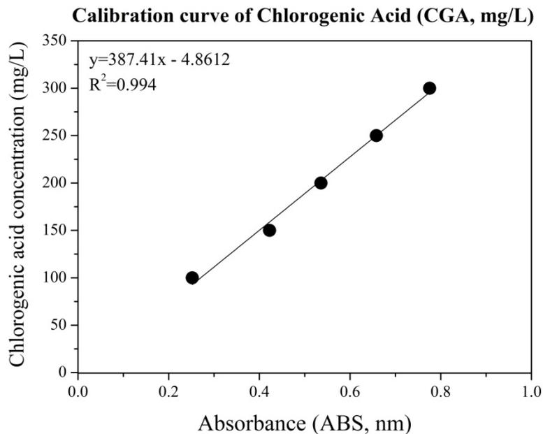
**Figure 4.12** Calibration curve of chlorogenic acid for the determination of total phenolic content
