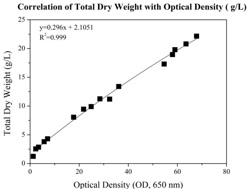
**Figure 4.9** Correlation curve of Total Dry Weight (TDW) with Optical Density (OD)
