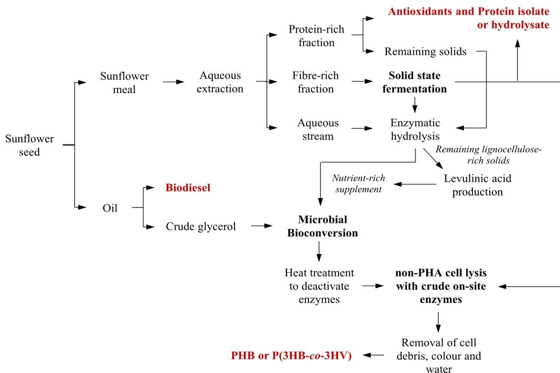
**Figure 10.1** Sunflower-based biorefinery concept for PHA production. Utilisation of SFM for the production of antioxidants, protein isolate and PHB or P(3HB-co-3HV)
