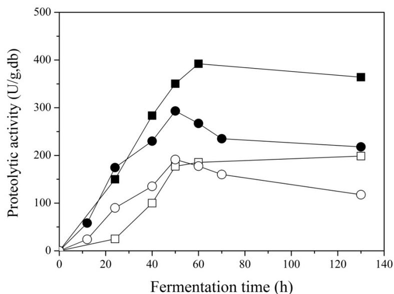
**Figure 5.5** Proteolytic activity during SSF with *A. oryzae* carried out at two different incubation temperatures with two different initial moisture contents (■: 65 % moisture
