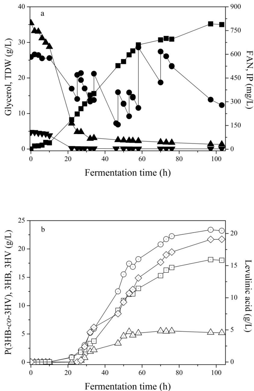
**Figure 7.3** Consumption of (▲) FAN, (●) glycerol and (▼) IP as well as production of (■) TDW, (○)P(3HB-co-3HV), (Δ) 3HV, (□) 3HB and (◇) LA during fed-batch bioreactor fermentation of *C. necator* on sunflower meal hydrolysate with feeding of crude glycerol and LA
