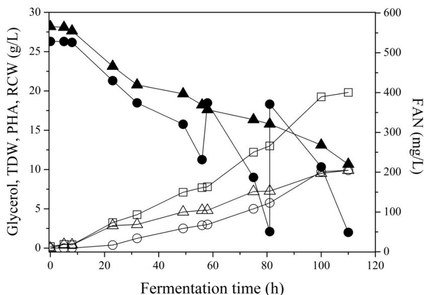
**Figure 6.2** Profile change of FAN (▲), glycerol (●), TDW (□), PHA (○) and RCW (△) during shake flask fermentation of *C. necator* DSM 545 on SFM hydrolysate and crude glycerol.
