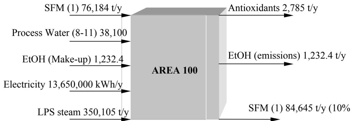
**Figure 10.3** Summary of total quantities of input and output streams employed in the extraction of the antioxidant-rich stream (AREA 100)
