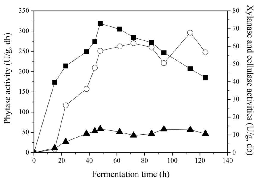
**Figure 5.6** Profile changes of phytase (■), xylanase (○) and cellulase (▲) during SSF carried out at 65 % (w/w) initial moisture content, uncontrolled pH and 30 °C
