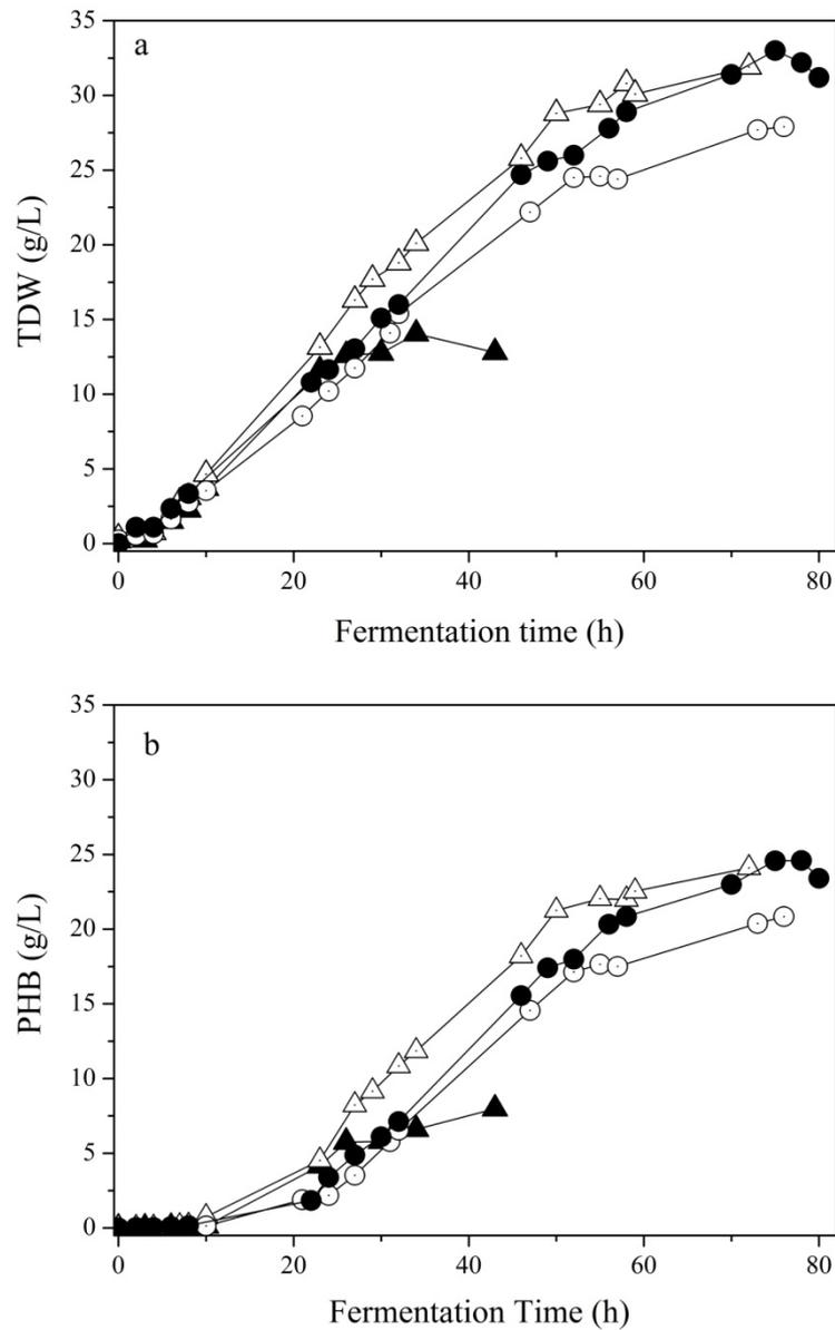
**Figure 6.5** TDW (a) and PHB (b) production during *C. necator* fed-batch bioreactor cultivations using sunflower meal hydrolysates and four different crude glycerol solutions including (▲) pure glycerol, (Δ) pure glycerol supplemented with inorganic chemicals, (○) original crude glycerol and (●) pre-treated crude glycerol via decanting
