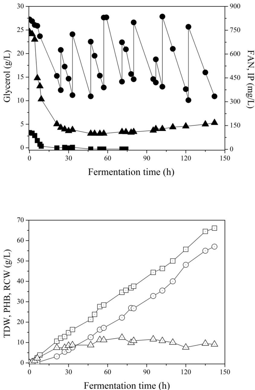
**Figure 8.11** Profile change of FAN (▲), glycerol (●), IP (■), TDW (□), PHB (○) and RCW (Δ) during batch bioreactor fermentation of *C. necator* cultivated on crude glycerol and Hydrolysate III
