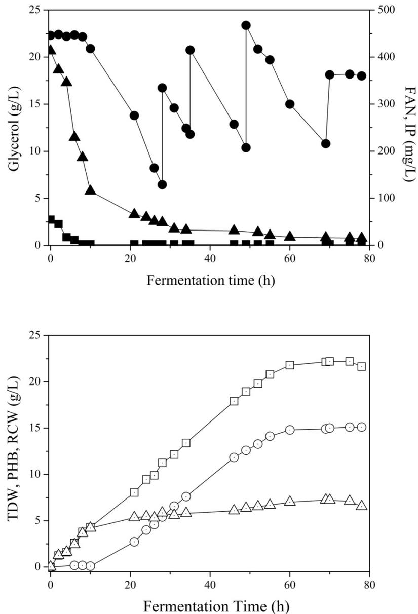
**Figure 6.6** Profile change of glycerol (●), FAN (▲), IP (■), TDW (□), PHB (○) and RCW (Δ) during fed-batch bioreactor fermentation of *C. necator* on sunflower meal hydrolysate with an initial FAN concentration of 412 mg/L (C/FAN ratio of 21.2 g/g)
