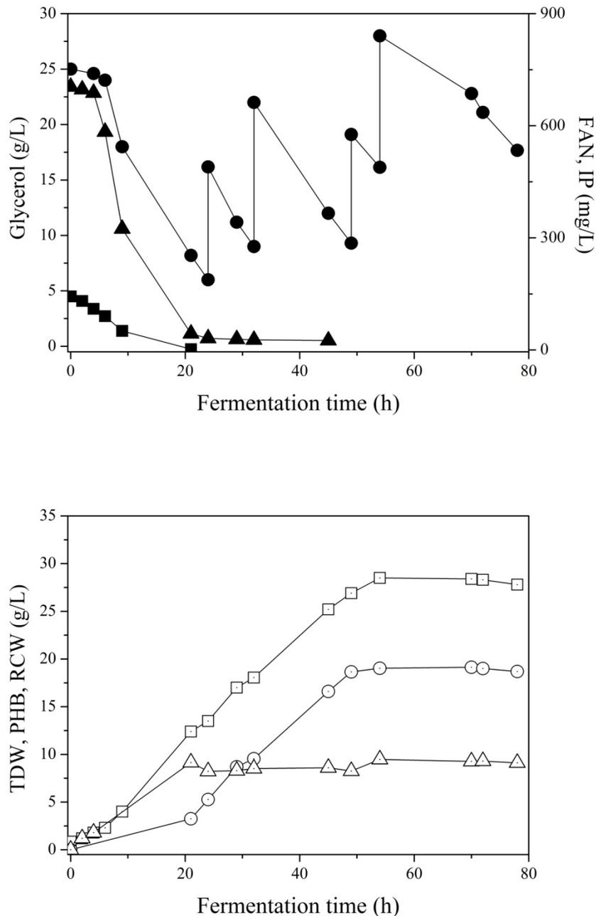
**Figure 8.10** Profile change of FAN (▲), glycerol (●), IP (■), TDW (□), PHB (○) and RCW (Δ) during batch bioreactor fermentation of *C. necator* cultivated on crude glycerol and Hydrolysate II
