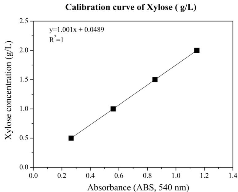
**Figure 4.6** Calibration curve of xylose
