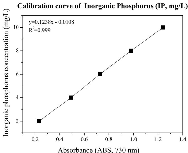
**Figure 4.4** Calibration curve of Inorganic Phosphorus (IP)
