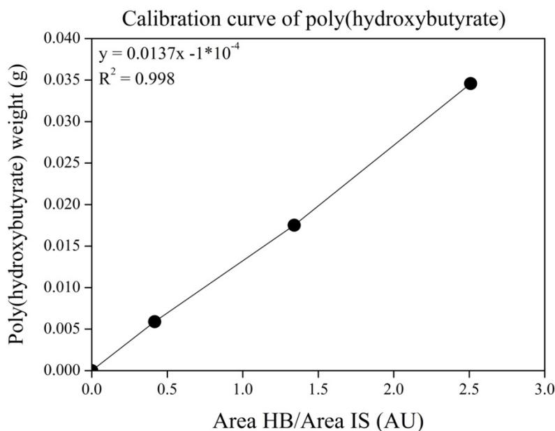
**Figure 4.10** Calibration curve of P(3-hydroxybutyrate) with internal standard (benzoic acid)
