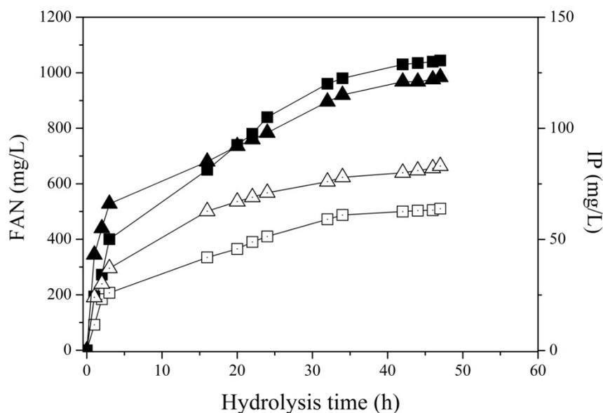
**Figure 8.8** FAN and IP production during enzymatic hydrolysis of 50 g/L ( $\square$ , FAN;  $\Delta$ , IP) and 100 g/L ( $\blacksquare$ , FAN;  $\blacktriangle$ , IP) initial concentration of solids using the solid residue fraction and the soluble fraction
