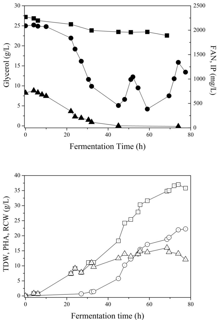
**Figure 6.9** Profile change of glycerol (●), FAN (▲), IP (■), TDW (□), PHB (○) and RCW (Δ) during fed-batch bioreactor fermentation of *C. necator* on sunflower meal hydrolysate with an initial IP concentration of 2 g/L
