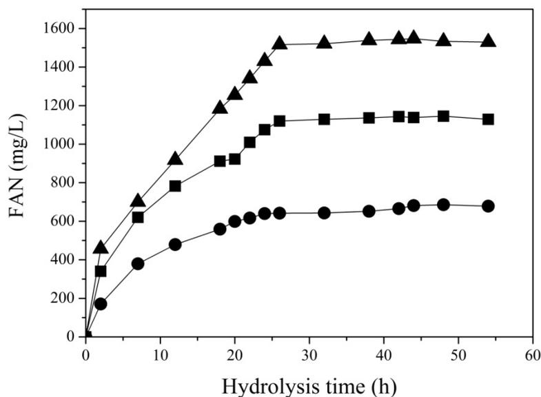
**Figure 5.10** FAN production during solid (SFM and remaining SSF solids) hydrolysis at initial solid concentrations of 46.3 g/L (●), 70.4 g/L (■) and 92.2 g/L (▲) using an initial enzyme activity of 6.4 U/mL
