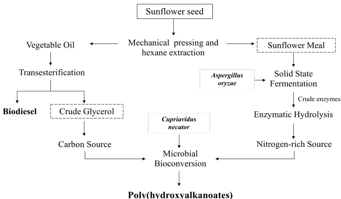
**Figure 2.6** Utilisation of sunflower-derived biodiesel industry by-products for PHA production
