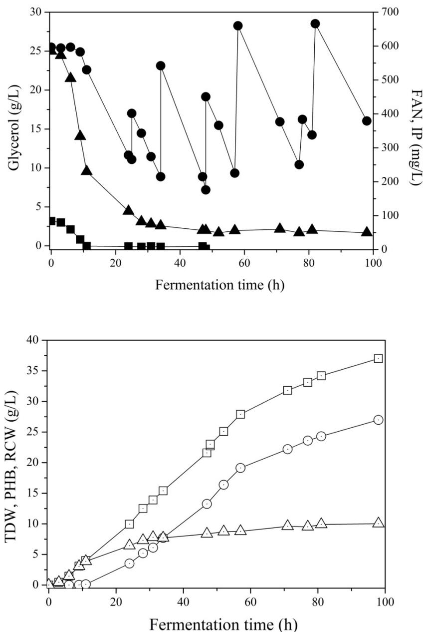
**Figure 6.7** Profile change of glycerol (●), FAN (▲), IP (■), TDW (□), PHB (○) and RCW (Δ) during fed-batch bioreactor fermentation of *C. necator* on sunflower meal hydrolysate with an initial FAN concentration of 585 mg/L (C/FAN ratio of 17.05 g/g)
