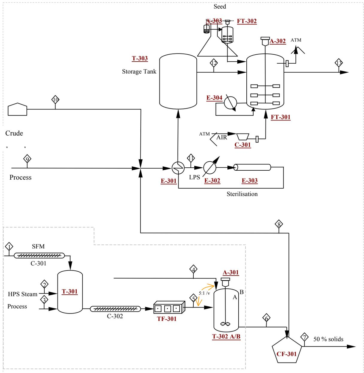
**Figure 10.6** Process flow diagram for AREA 300: solid state fermentation, enzymatic hydrolysis and PHB production via fermentation
