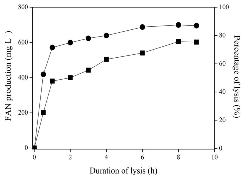
**Figure 9.6** FAN production (■) and percentage of non-PHA cell lysis (●) during enzymatic lysis of 50.1 g/L initial TDW using crude enzymes produced by *A. oryzae*
