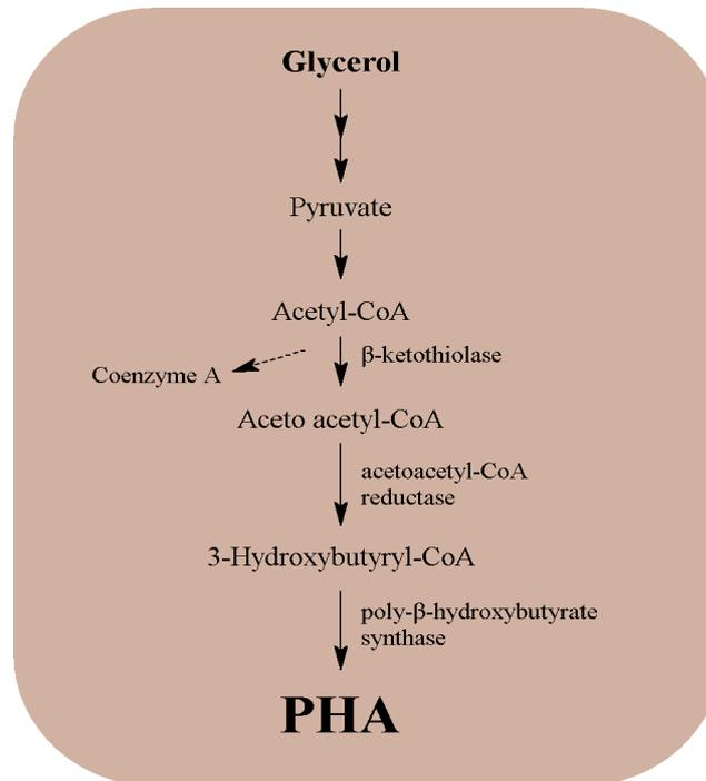
**Figure 2.5** PHB biosynthetic pathway of *Cupriavidus necator* from glycerol
