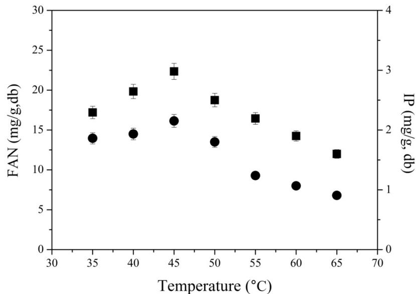
**Figure 5.8** Effect of temperature on FAN (●) and IP (■) production during hydrolysis of 45 g/L initial solid (SFM and remaining SSF solids) concentration using an initial enzyme activity of 6.4 U/mL
