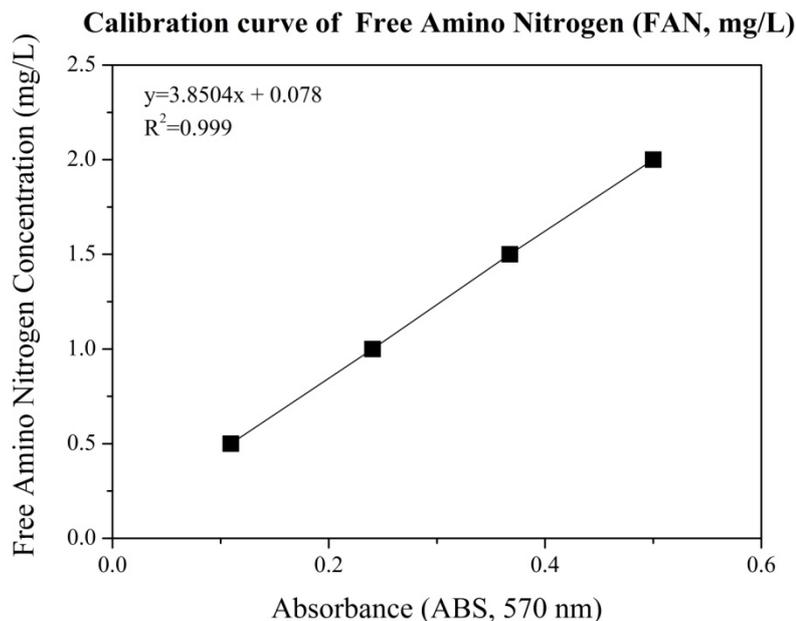
**Figure 4.3** Calibration curve of free amino nitrogen (FAN)
