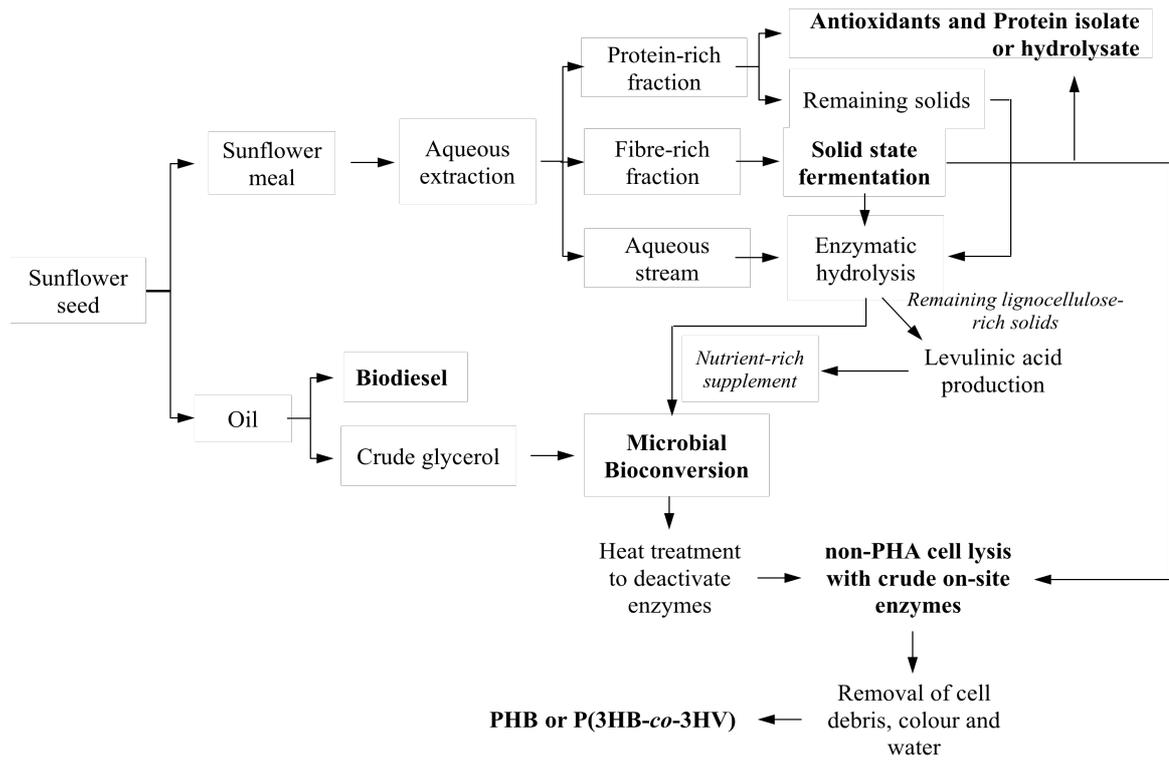
**Figure 4.13** Sunflower-based biorefinery concepts for PHA production. Utilisation of SFM for the production of antioxidants, protein isolate and PHB or P(3HB-co-3HV)
