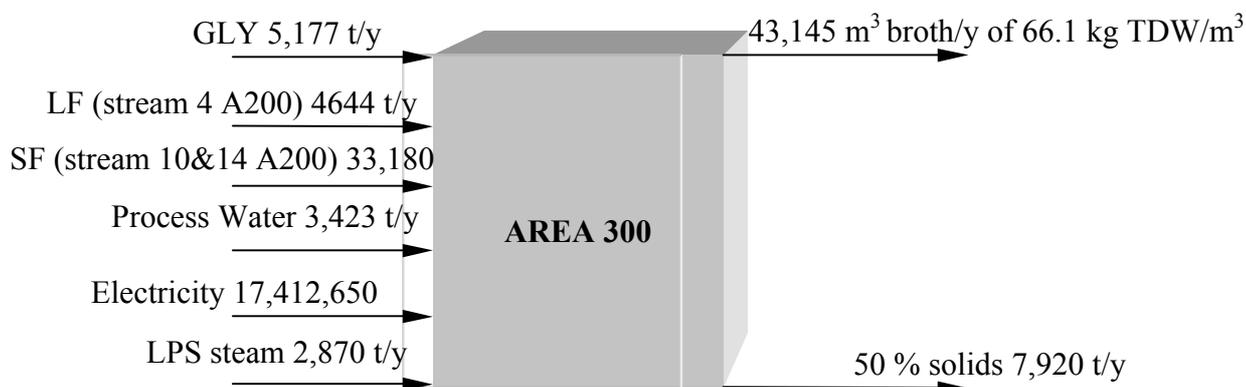
**Figure 10.7** Summary of total quantities of input and output streams during solid state fermentation, enzymatic hydrolysis and fermentation (AREA 300)
