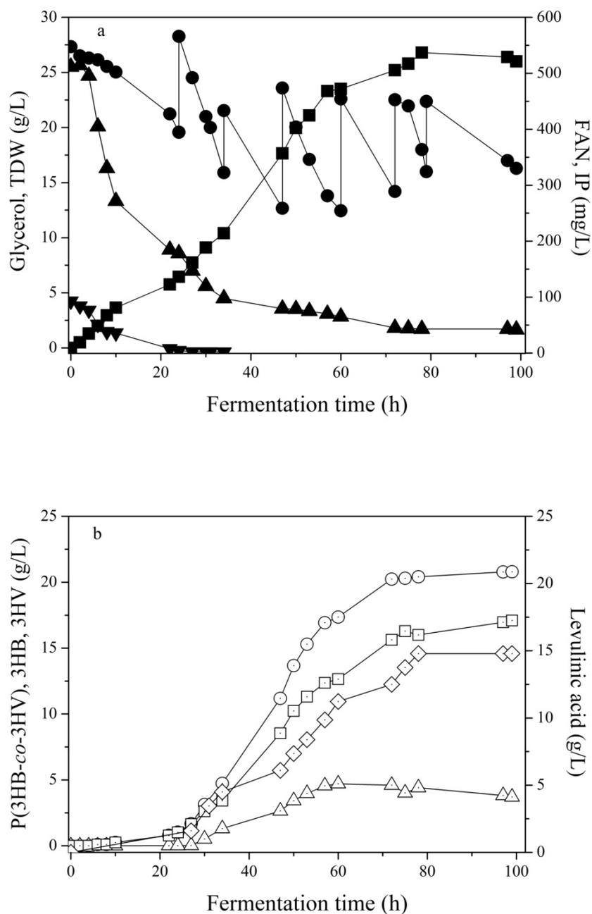
**Figure 7.2** Consumption of (▲) FAN, (●) glycerol and (▼) IP as well as production of (■) TDW, (○) P(3HB-co-3HV), (Δ) 3HV, (□) 3HB and (◇) LA during fed-batch bioreactor fermentation of *C. necator* on sunflower meal hydrolysate with feeding of crude glycerol and LA
