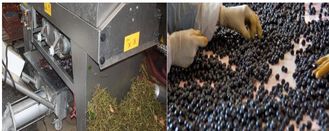
Figure 3.2: Destemming process: separation of stalks or stems mechanically and manually ( www.aubaimema.com/en/about-vinification.html (image on the left side), www.smith-haut-lafitte.com/en/smith-haut-lafitte-bio-precision.html (image on the right side), accessed 09/2015)
