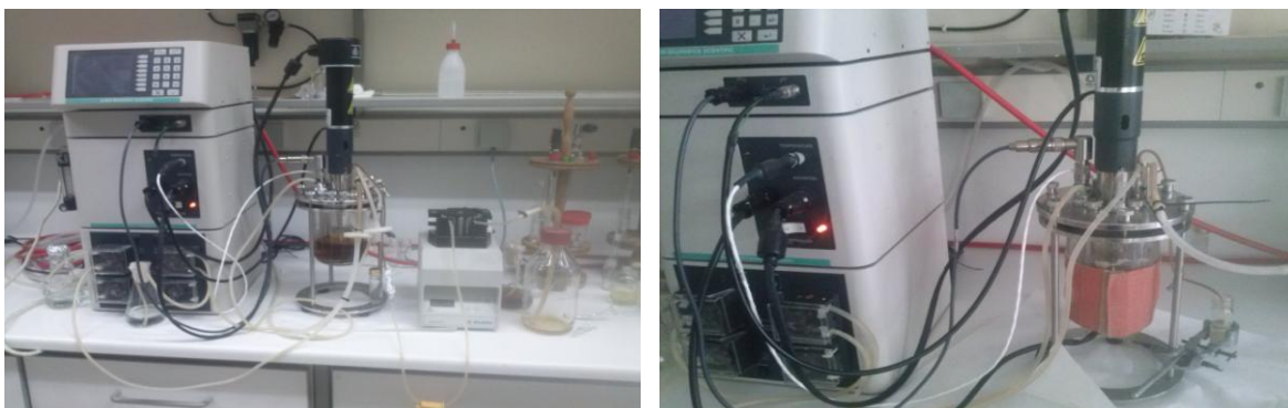
Figure 6.6: The lab-scale bioreactor used in the fermentations for PHB production (New Brunswick Scientific Co, USA)
