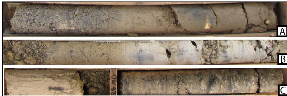
Figure 5-1. Images from the drilled cores. (A) Borehole GA-4 from 18.30 m till 19.20 m, showing the transition from fluvial (gravels) to marine (silt). (B) Borehole GA-4 from 33.00 m to 33.90 m, showing the transition from gravels to silty sand. (C) Borehole GA-5 from 28.60 m to 29.70 m, showing the transition from marine (clayey sand) to fluvial gravels.
