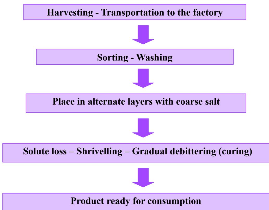
**Figure 1.3.** Flow diagram for the processing of natural black olives in dry salt.
