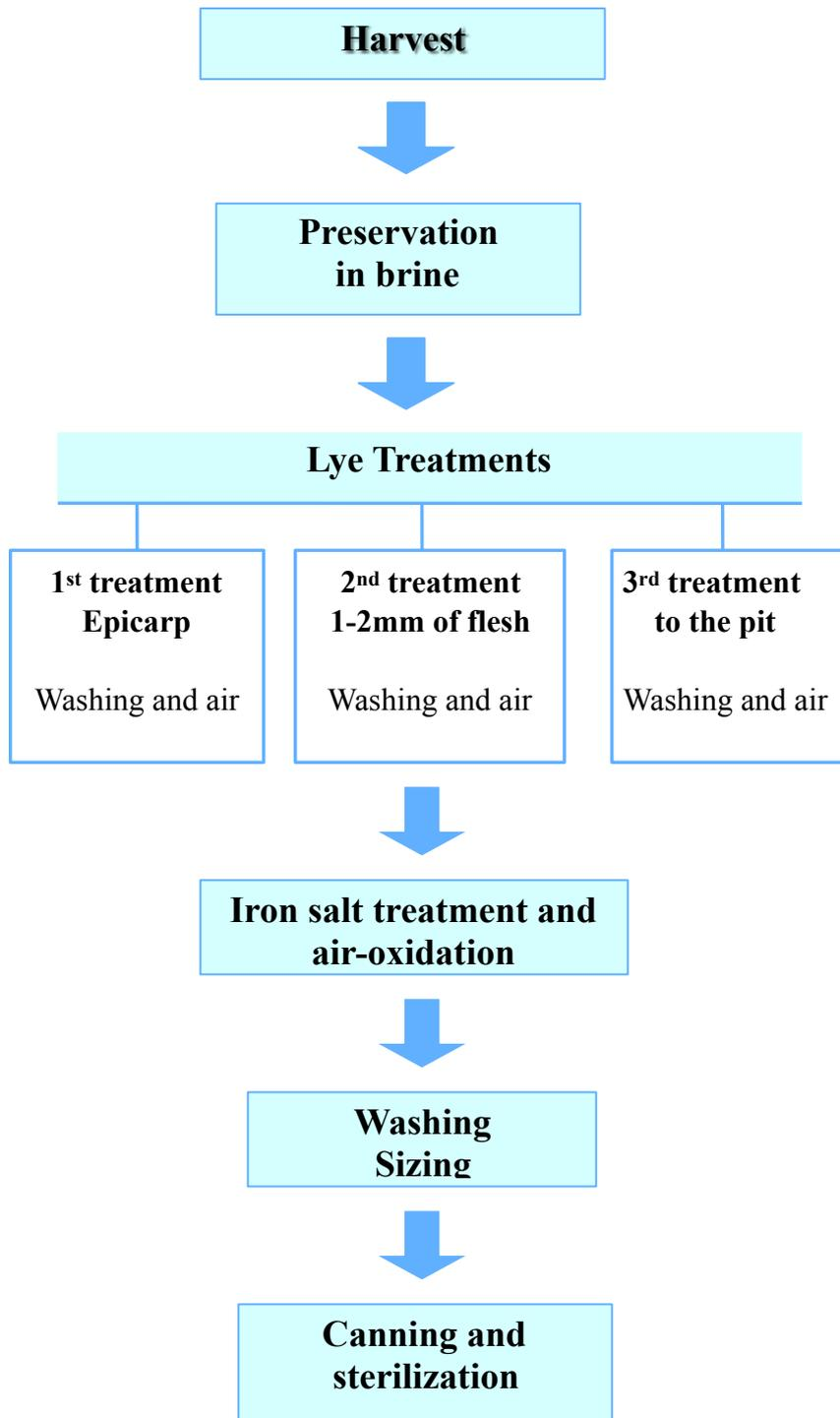
**Figure 1.4.** Flow diagram for the processing of Californian-style black ripe olives (adapted from Marsilio et al. 2001b).
