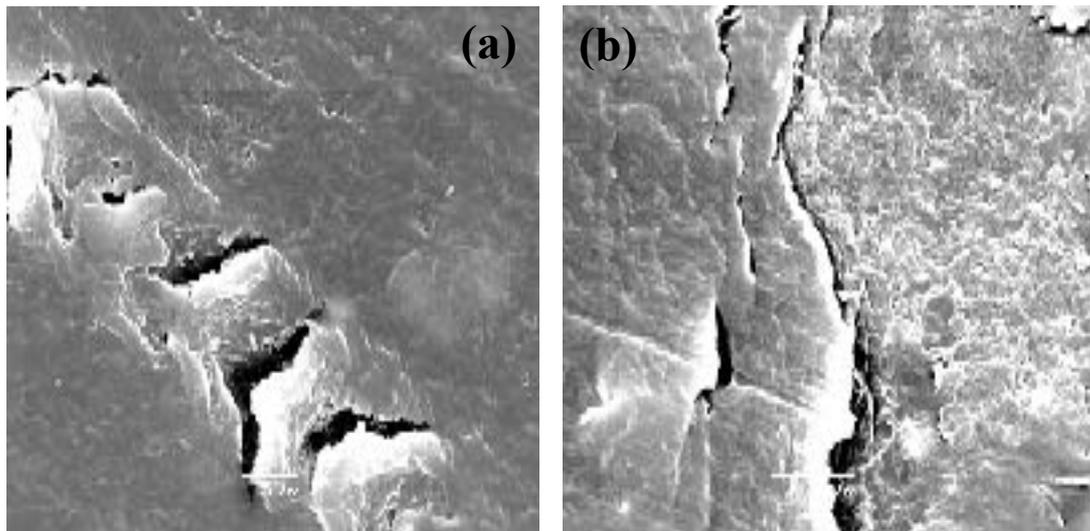
**Figure 5.2.** Scanning Electron Microscopy (SEM) microphotographs of the fermentation vessels from the middle (a) and upper (b) sampling spots after treatment B after 60 days.
