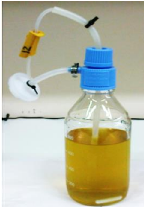
Figure 2.1. Anaerobic batch fermentation in 1-l Duran bottle (The photo was taken in the laboratory).
