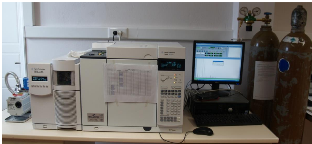
Fig 2.1.: GC/MS instrument utilized in the PhD thesis
