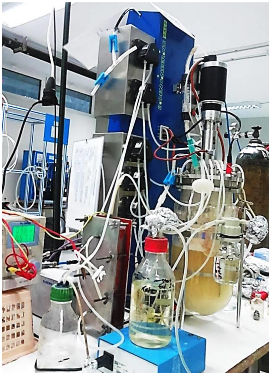
Figure 4.5 Integrated succinic acid production and separation using an electrochemical bioreactor
