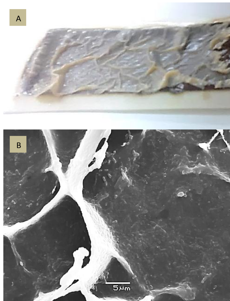
Figure 8.9 (A) Biofilm formation on the anionic membrane. (B) B. succiniciproducens cells on the biofilm observed with scanning electron microscope (SEM)
