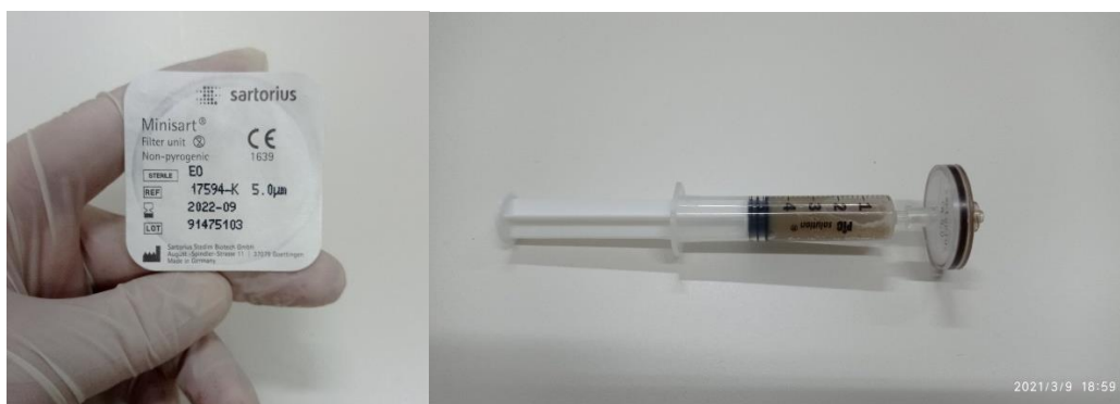
Figure 11. “Sample filtering using 5.0 µm filter and syringe prior to testing with the novel diagnostic device.”
