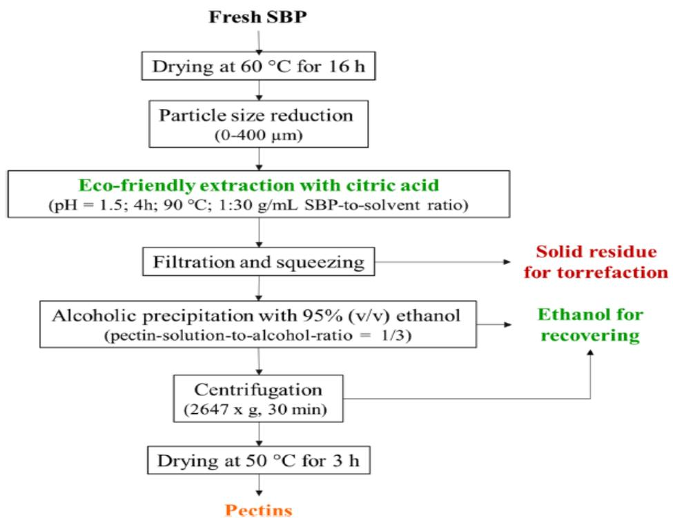
**Figure 11.** A simplified laboratory process flowchart outlining a streamlined biorefinery approach for converting SBP into valuable commodity chemicals and solid fuels (Adiletta et al., 2020).
