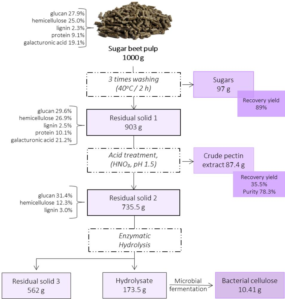
**Figure 24.** Mass balances and proposed process for the SBP biorefinery.
