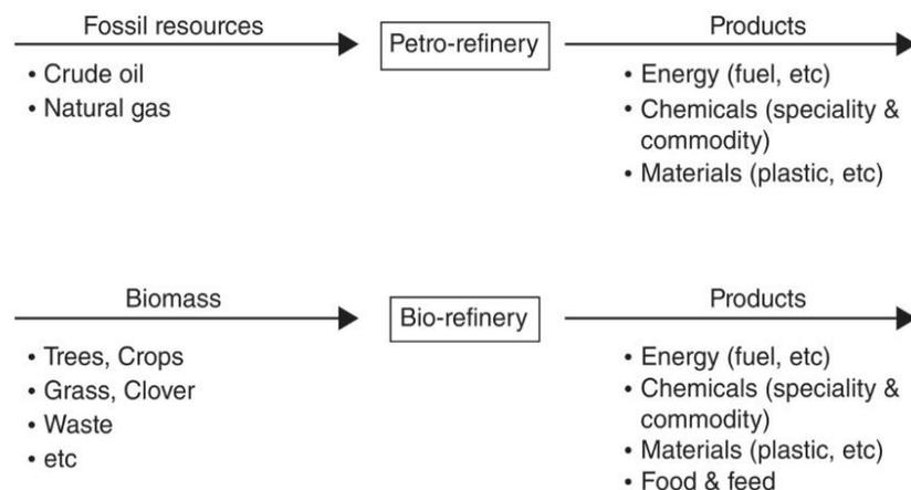
**Figure 7.** Comparison of biorefinery vs petrorefinery (Clark & Deswarte, 2015).
