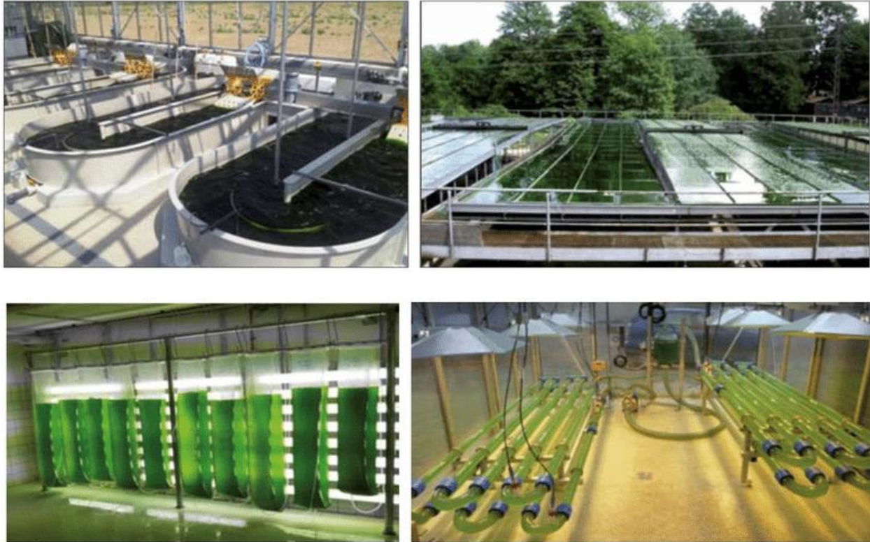
Closed cultivation systems for cultivation of microalgae; left: sleeve-bag photobioreactor; right: tubular photobioreactor
