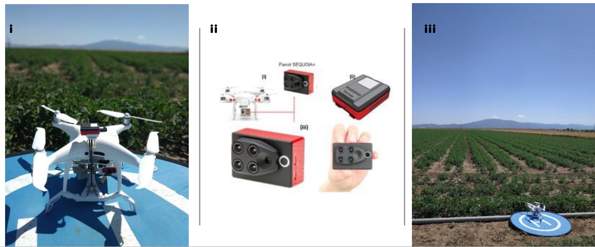
Figure 26. i) a Phantom 4 Pro UAS used to collect imagery, ii) Parrot Sequoia+ multispectral camera of the UAS, iii) On site data collection
