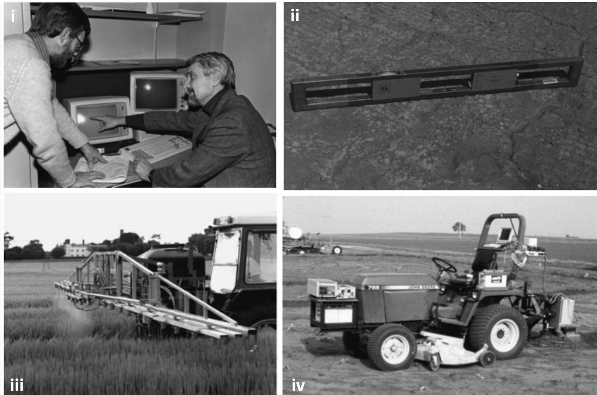
Figure 2. i) Pierre Robert explaining his computerized farming by soil map database (1985) to Jim Anderson at the University of Minnesota, ii) First commercial unit (1980) of the Geonics EM-38 single dipole electromagnetic induction conductivity meter, iii) Variable rate herbicide applicator developed by Stafford and Miller (1993), iv) Soil organic matter sensor based on NIR reflectance (1991). Source: [36].
