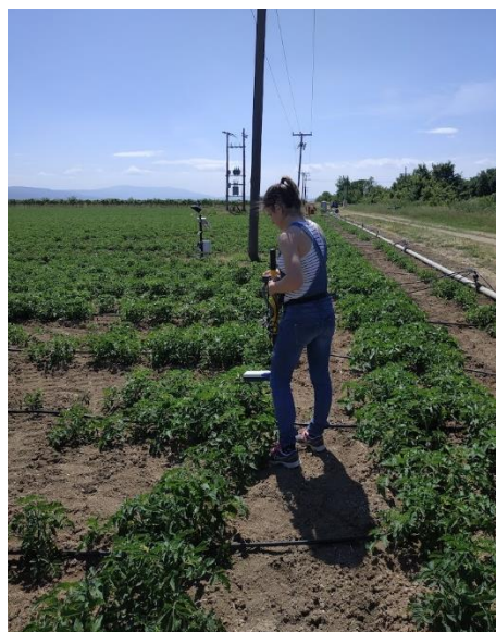
Figure 27 : GreenSeeker hand-held optical sensor. Source: Personal Archive
