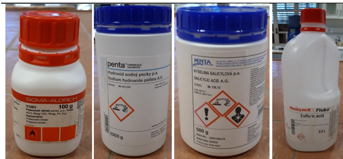
Figure 18: Reagents for the colorimetric determination of the nitrate-nitrogen through the nitration of salicylic acid
