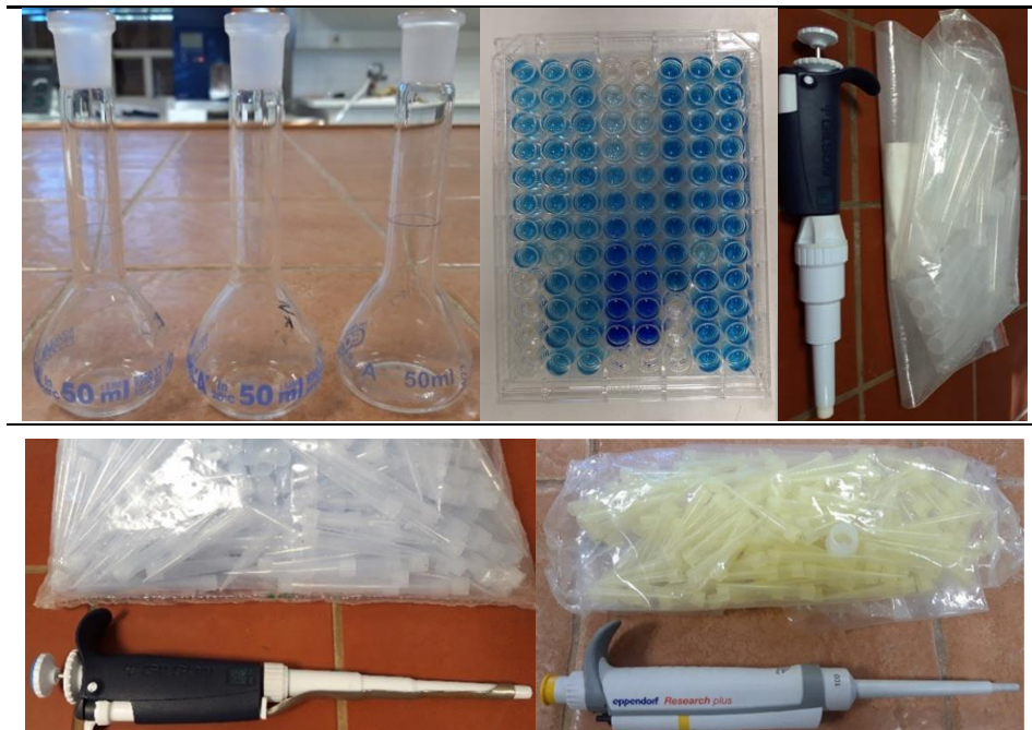
Figure 14: Materials used for the molybdenum blue reaction for orthophosphate determination
