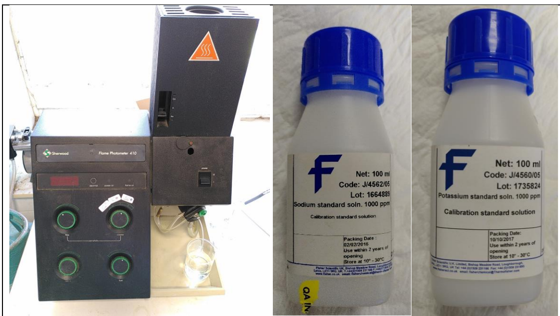
Figure 20: Flame Photometer by Sherwood and standard solution for the preparation of the calibration curve
