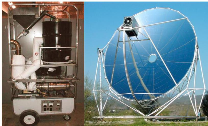
Figure 2.9 - Micro-Biomass Stirling CHP and Solar Euro-Dish Stirling Concentrator
