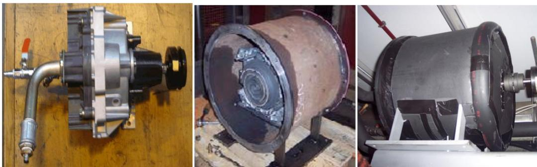
*Figure 6.5 - The open-drive oil-free air compressor*
